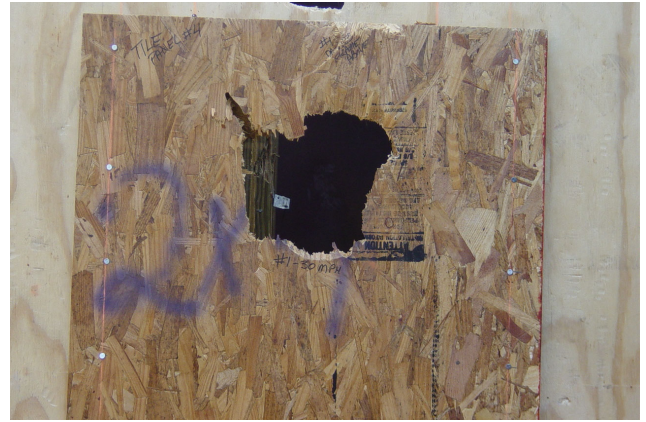
Figure 2-4. Typical 6.6 lb. Clay Tile Impact on OSB Panel
