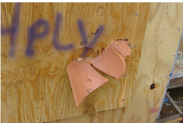
Figure 2-3. Typical 6.6 lb. Clay Tile Impact on Plywood Panel
