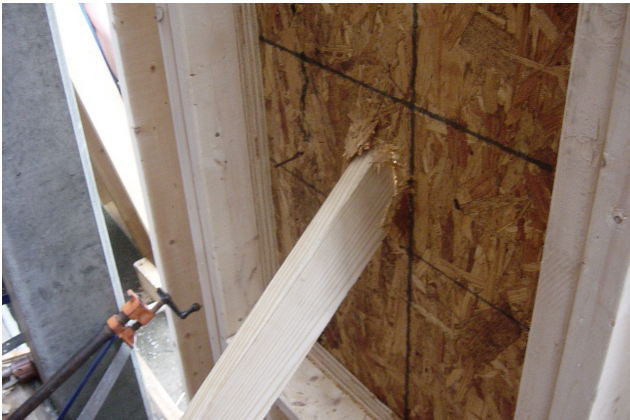
Figure 2-2. Typical 4.5 lb. 2x4 Missile Impact on OSB Panel.
