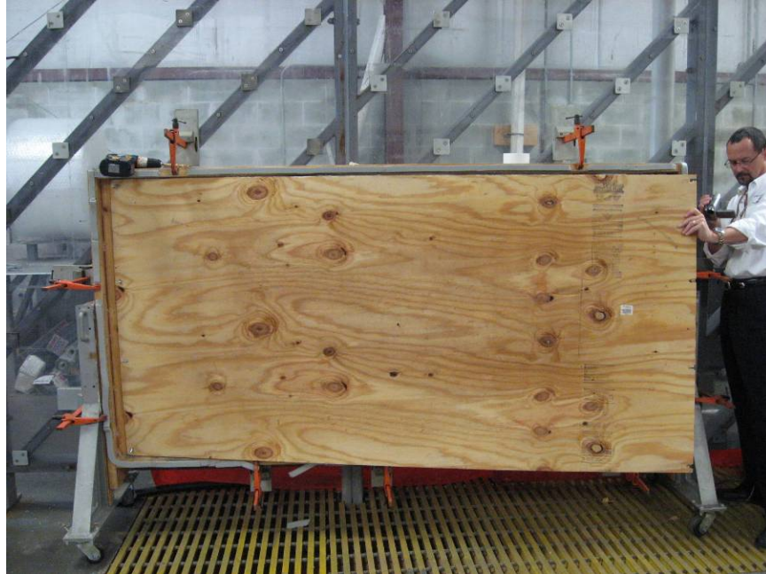
Photo No. 1 Specimen # 1 1/2" CDX plywood with 16" on center spacing; test specimen after structural loading
