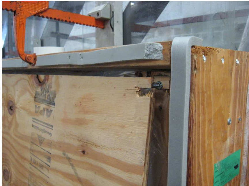
Photo No. 2 Specimen # 1 Failure on right side at 33.2psf
