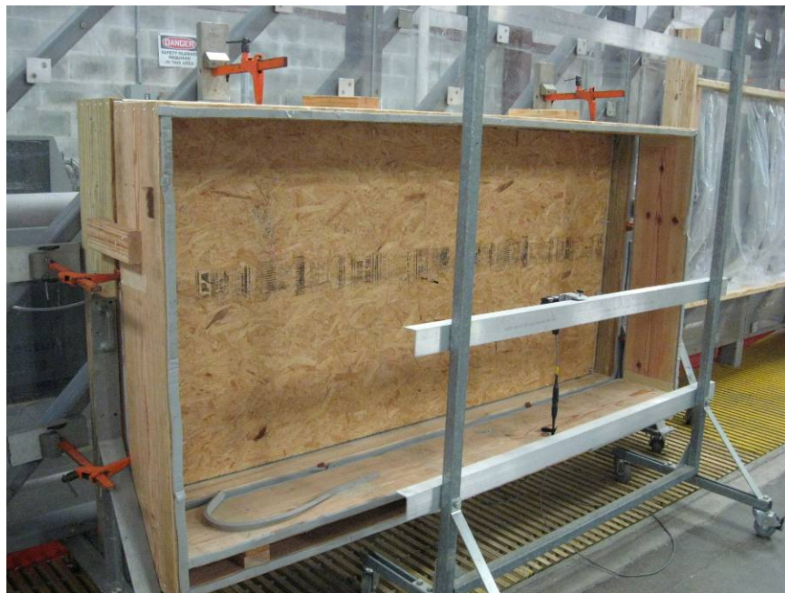
Photo No. 4 Specimen # 2 7/16" OSB with 16" on center spacing
