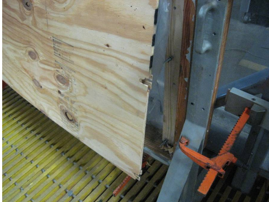
Photo No. 3 Specimen # 1 Failure on right side at 33.2psf
