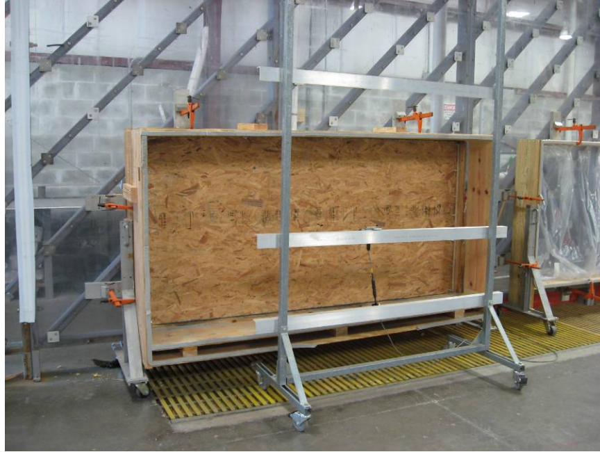
Photo No. 7 Specimen # 3 7/16" OSB with 8" on center spacing
