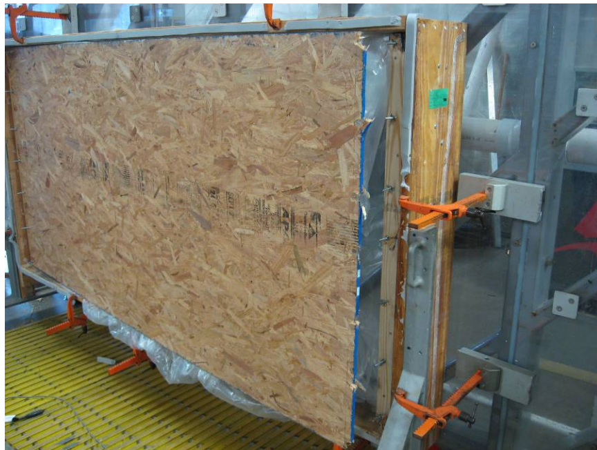
Photo No. 8 Specimen # 3 Failure on right side at 52.6psf
