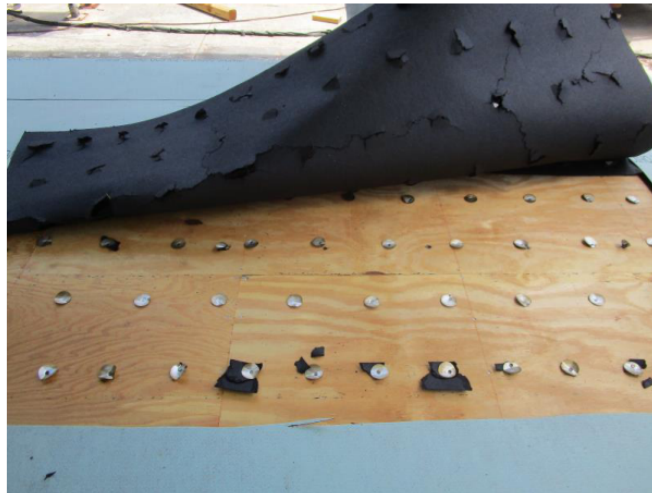
Specimen #2 failure – fastener pull-through
