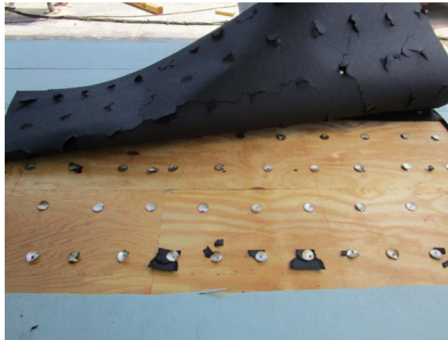
Specimen #2 failure – fastener pull-through
