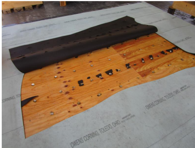
Specimen #4 failure – fastener pull-through
