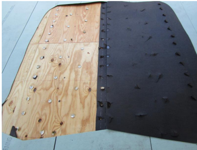
Specimen #1 failure – fastener pull-through
