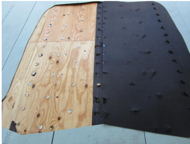
Specimen #1 failure – fastener pull-through
