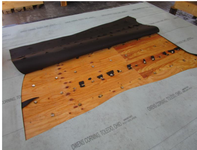
Specimen #4 failure – fastener pull-through
