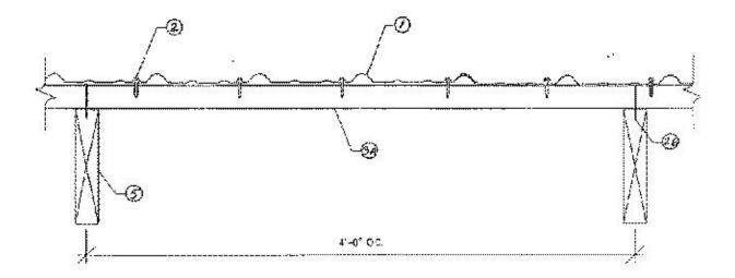
1. **Metal Roof Deck Panels\*** — No. 29 MSG min coated steel. Max panel width 36 in Rib height max 3/4 in. Panels continuous over two or more spans. Panels to overlap 6 in. at endlaps and must occur adjacent to a support when plywood decking (Item 3) is not used. A bead of sealant may be used at panel endlaps and sidelaps.
