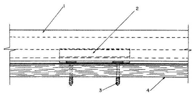
1. **Metal Roof Deck Panels\*** — 0.032 in. thick aluminum or No. 24 MSG coated steel, 16 in. wide, 1-3/8 in. high at the male rib. Panels continuous over two or more spans.
