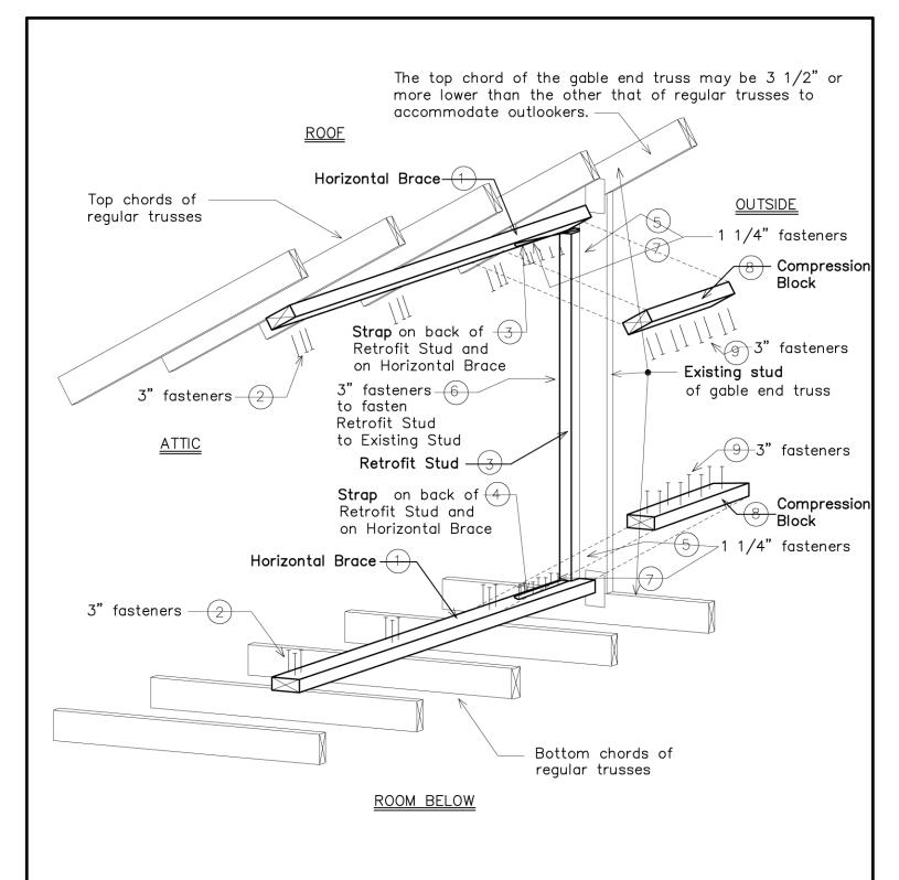
The gable end shown is a truss gable end. Similar retrofit measures apply to conventionally framed gable ends.
