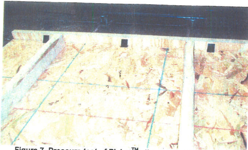
Figure 7. Pressure test of Plylox™ clips with 8 ft panel span and 2-2x4 stiffeners.
