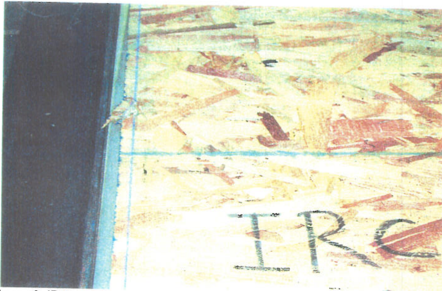
Figure 3. IRC panel specimen (nominal 8 ft opening span) showing pull-thru and edge tear-out of one #8 screw at one end of the panel.
