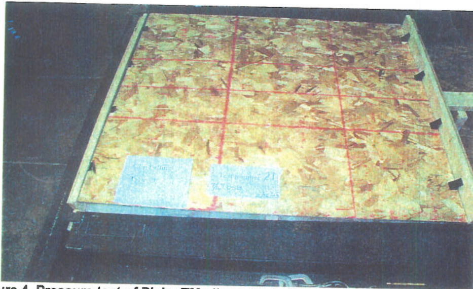
Figure 4. Pressure test of Plylox™ clips with 1x10 wood opening recess material (Specimen #21, nominal 4 ft x 4ft panel, failure by clip bend on left side).
