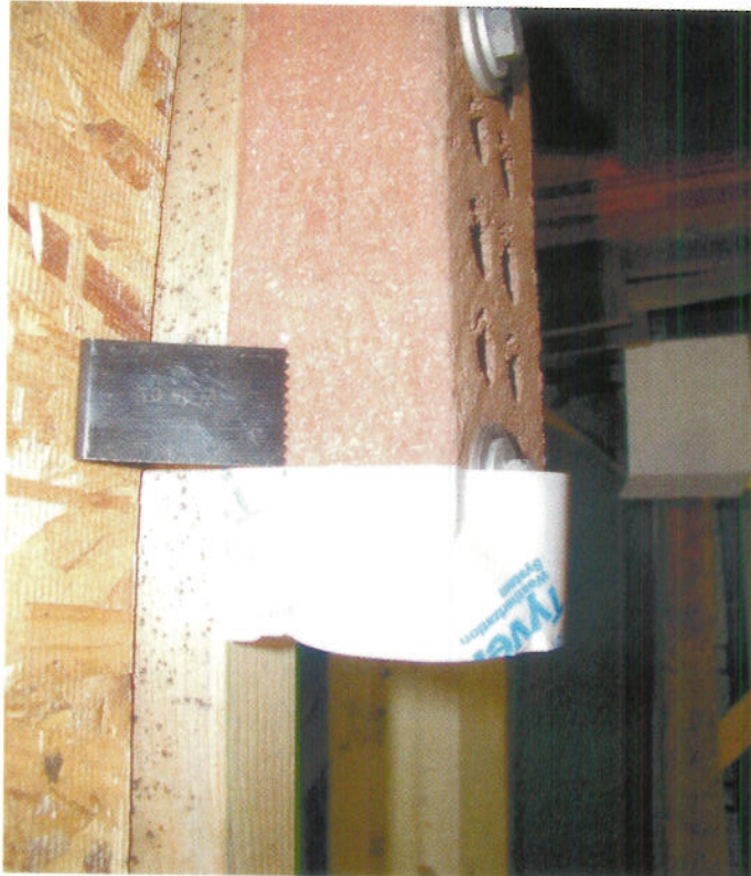
Figure 4. Clip attachment detail (Mark (not visible in the photo) on the Tyvek tape was used to monitor location of the clip).
