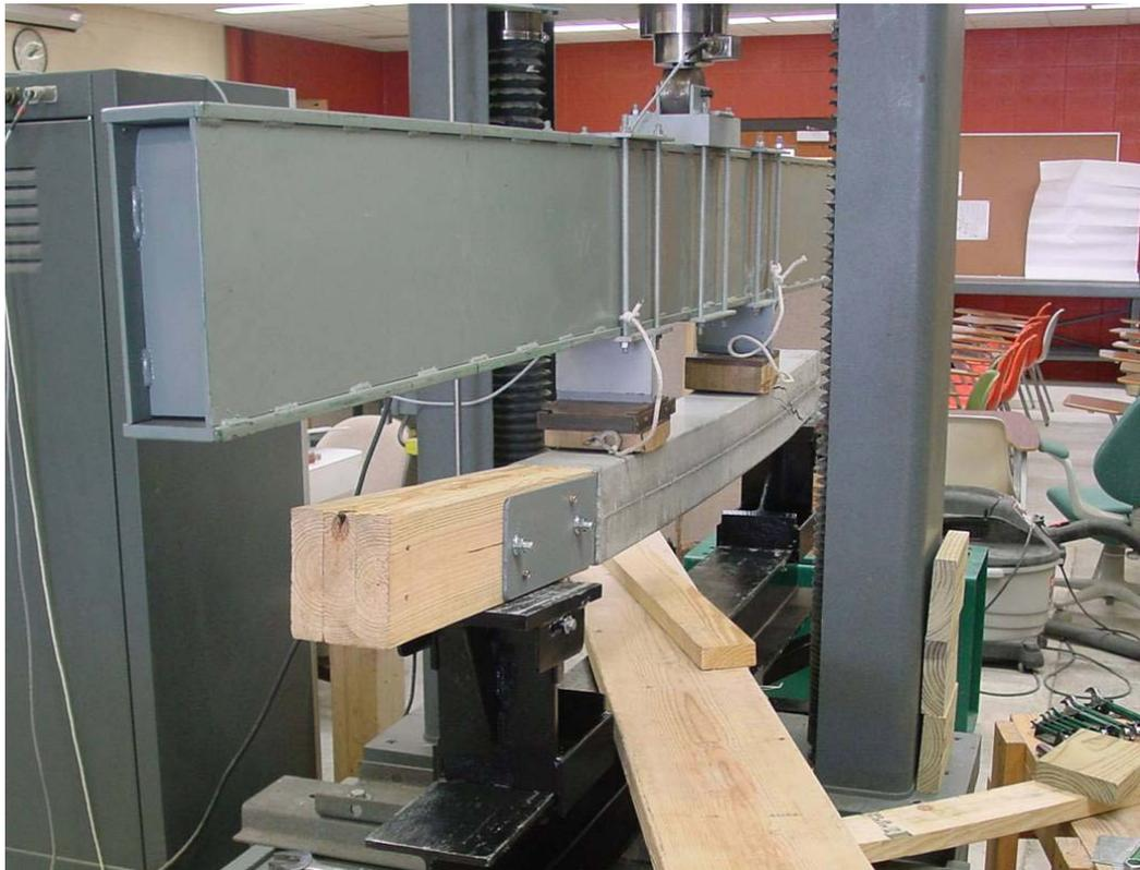
Figure C.2. Load application with a Tinius Olson Universal Compression-Tension Testing Machine.
