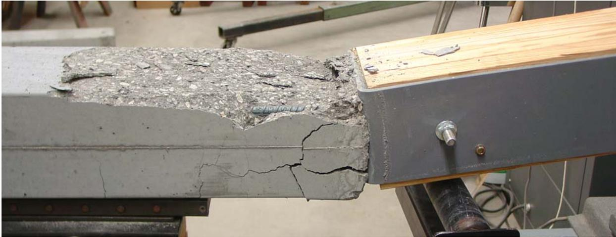
Figure B.5. Typical bending failure mode for steel bracket-to-concrete connection.
