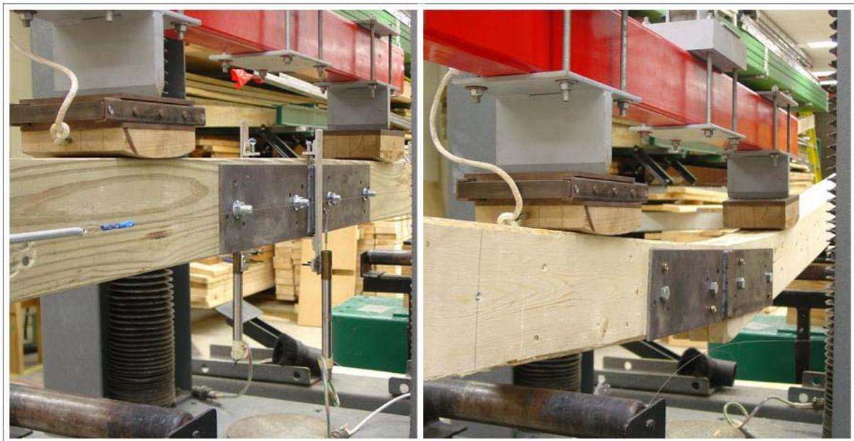
Figure D.5. Bolted connection prior to testing showing placement of wire deflectometers (left) and combo connection (connection with bolts and SDS screws) at maximum load (right).
