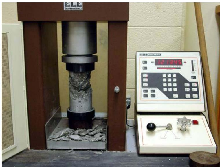
Figure C.4. Compressive strength testing of concrete used in shear test specimens.
