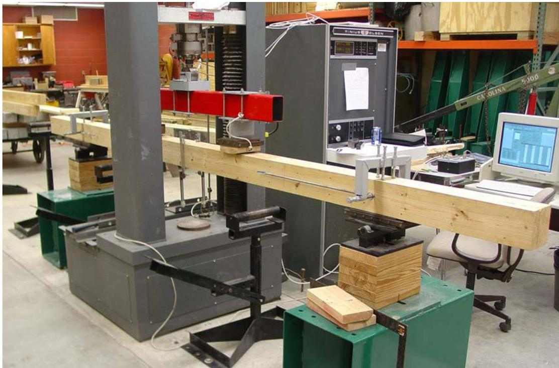
Figure D.3. Test set-up for determination of lumber modulus of elasticity.
