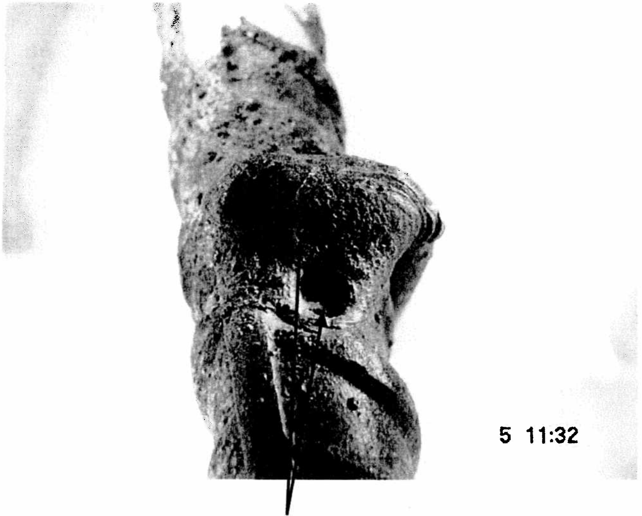
Specimen # 9, Location # 2 Voids/ Surface porosity in Fillet weld created by gas pocket coming to surface
