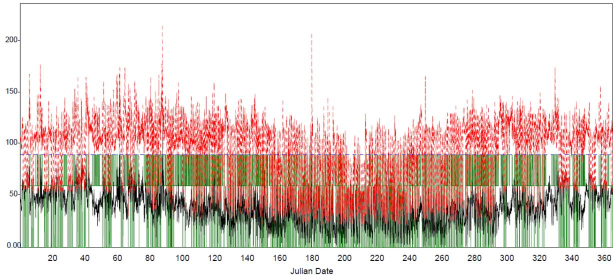
**Figure Ex-1. Tallahassee balanced system with outdoor temperature-based smart ventilation showing infiltration airflow in black and the total airflow in red including the varying mechanical ventilation in green. Fan ventilates at 0, 60 or 90 cfm based on outdoor temperature. Goal is to achieve an annual average of 90 cfm per ASHRAE 62.2-2013 total outside air requirements (blue dashed line).**
