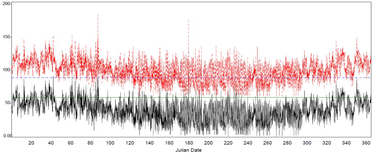
**Figure 14. Tallahassee balanced system airflow showing the infiltration in black and the total airflow in red including the constant 60 cfm of mechanical ventilation (green line) designed to achieve the 90 cfm ASHRAE 62.2-2013 goal (blue dashed line).**
