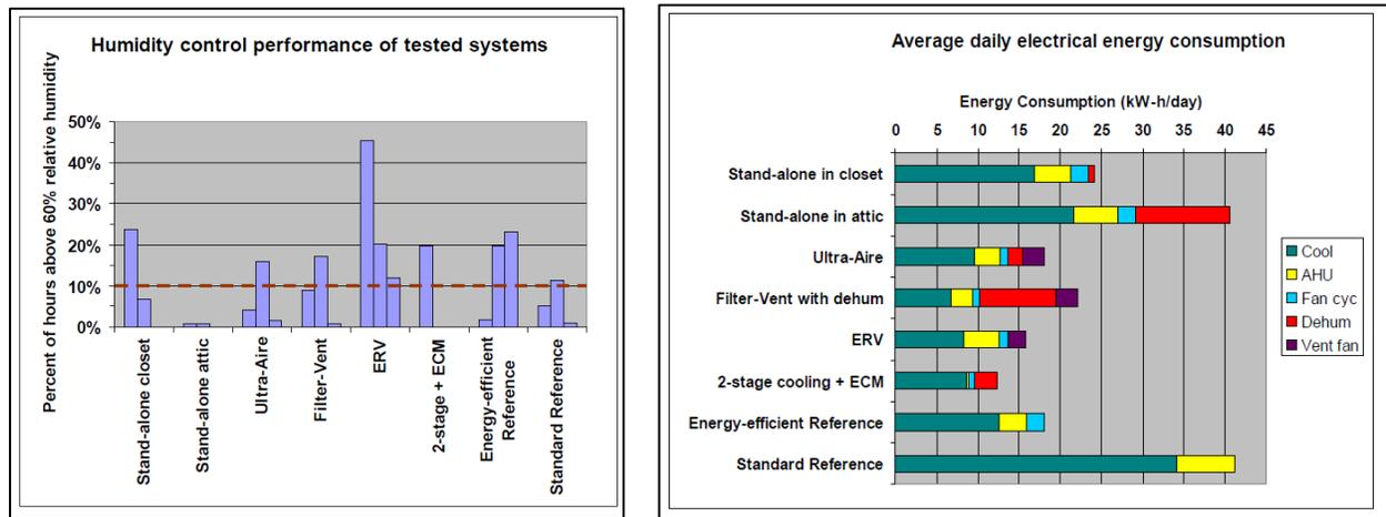
**Figure 3. Humidity frequencies and electrical use in homes with six different dehumidification strategies (from Armin Rudd, Joseph Lstiburek, Kohta Ueno, “Residential Dehumidification Systems Research for Hot-Humid Climates,” Figures 10 & 14).**
