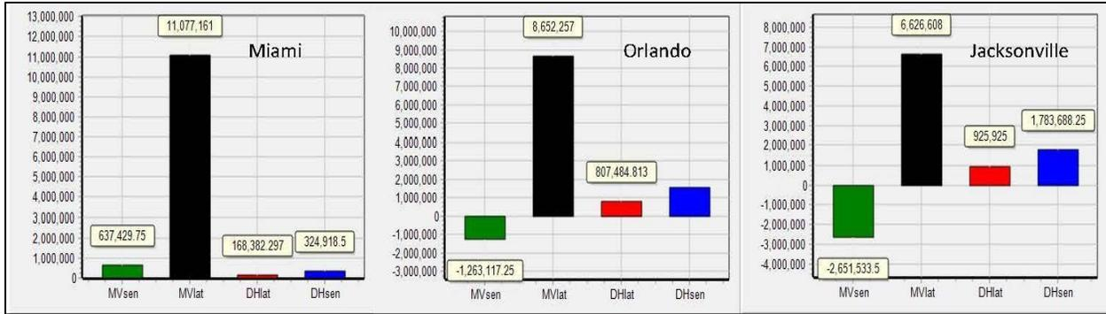
**Figure 11 Annual (Btu/year) mechanical venting added latent and sensible loads and dehumidifier removed latent load and added sensible load.**
