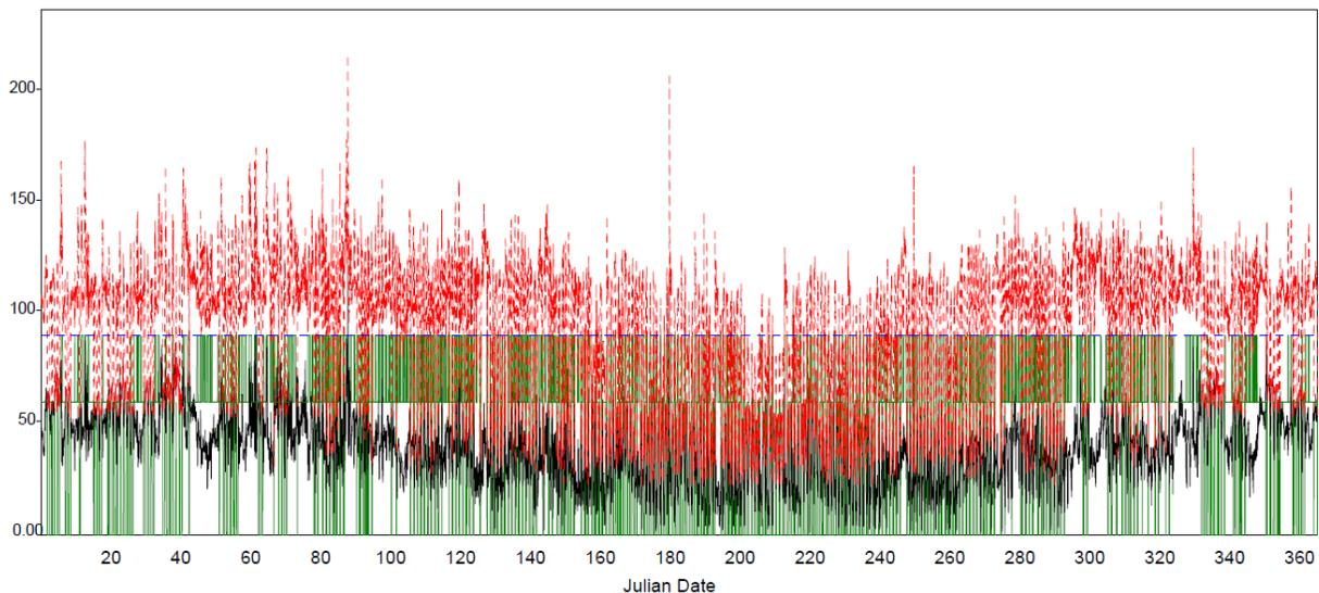
**Figure 15. Tallahassee balanced system with outdoor temperature-based smart ventilation showing infiltration airflow in black and the total airflow in red including the varying mechanical ventilation in green. Fan ventilates at 0, 60 or 90 cfm based on outdoor temperature. Goal is to achieve an annual average of 90 cfm per ASHRAE 62.2-2013 total outside air requirements (blue dashed line).**
