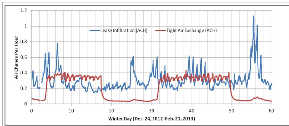
**Figure 4. Winter measured air exchange between leaky 8ACH50 home (Blue line) and tight 2ACH50 home (Red line). Tight home ran for two weeks with 63 cfm of supply ventilation air and then was 0 ventilation for two weeks.**
