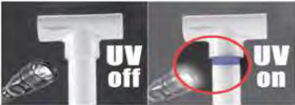
Inspector can verify the use of Primer with a UV flashlight.
