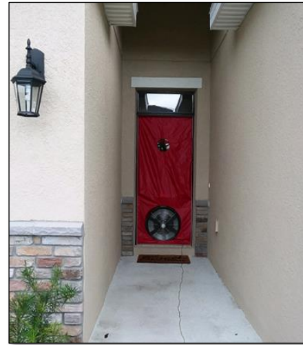
Figure 1. Blower door set-up at study home.
