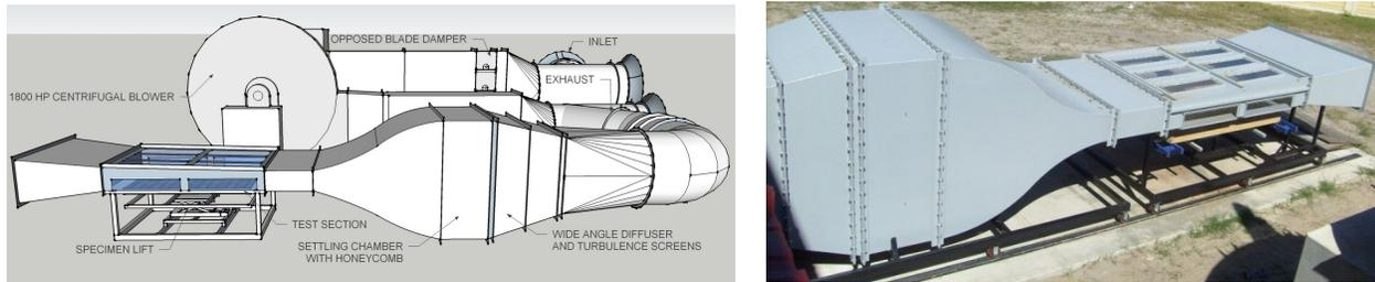
**Figure 1.** Dynamic Flow Simulator a) componentry and b) as constructed.
