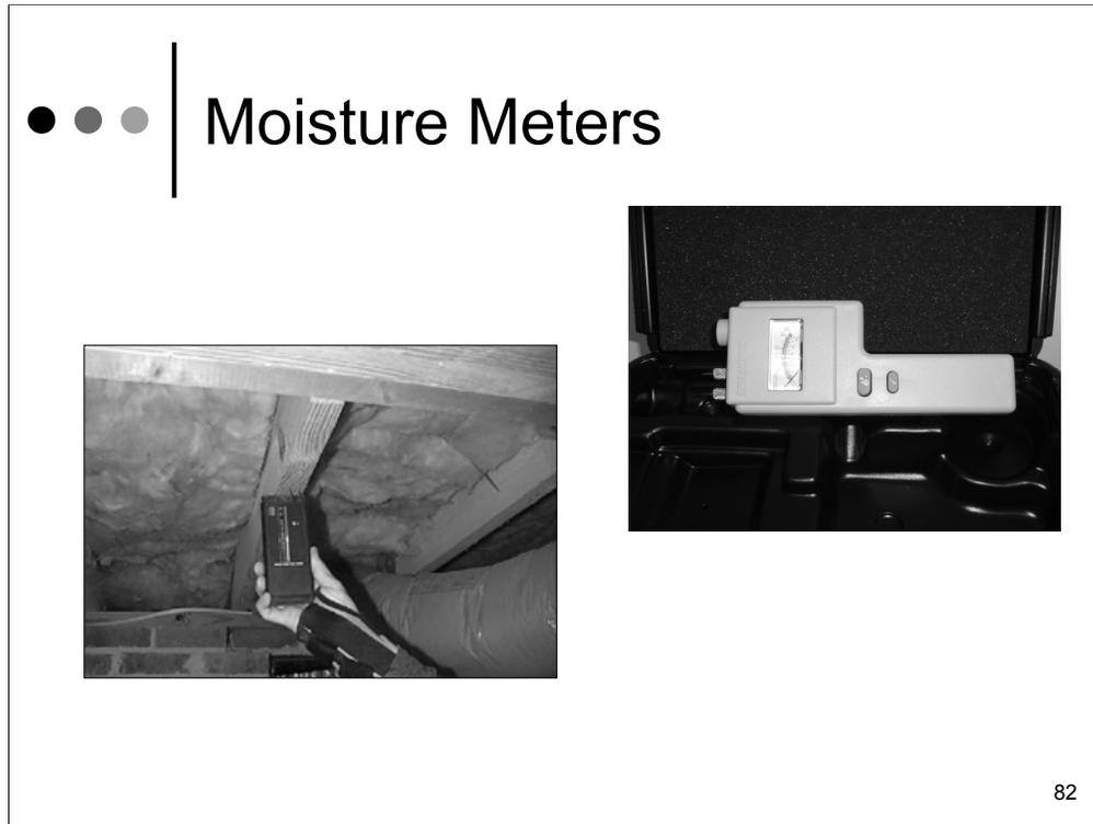
Some moisture meters are only calibrated for wood, but may be suitable for measuring moisture levels in other non-conductive materials. The following descriptions are general in nature and may not be accurate for the moisture meter you purchase. Be certain to carefully read all directions before purchasing.
