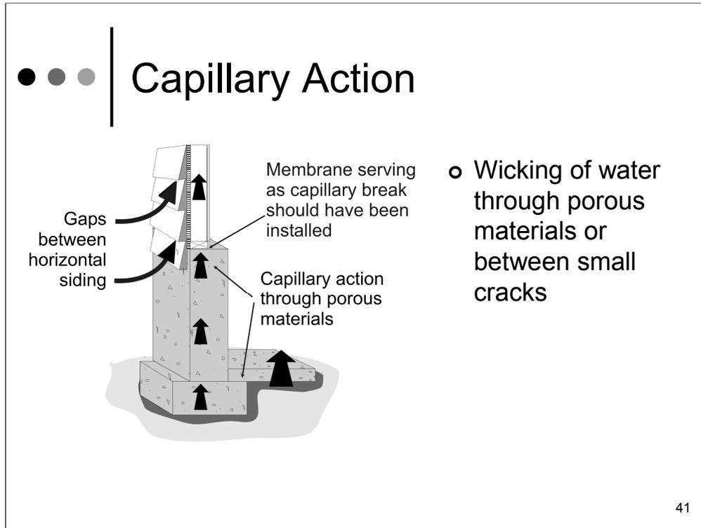
Capillary action can be caused by water seeping between overlapping pieces of exterior siding; by water drawn upward through pores or cracks in concrete slabs; and by water migrating from crawl spaces into attics through foundation walls and wall framing.
