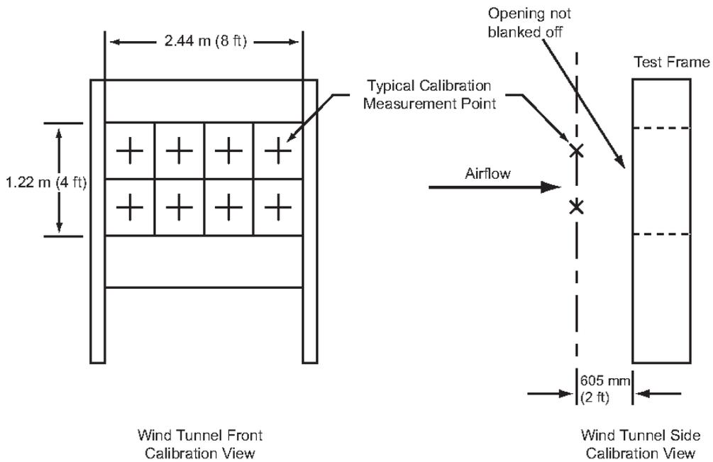
Figure 3 - Wind Stream Calibration Setup
