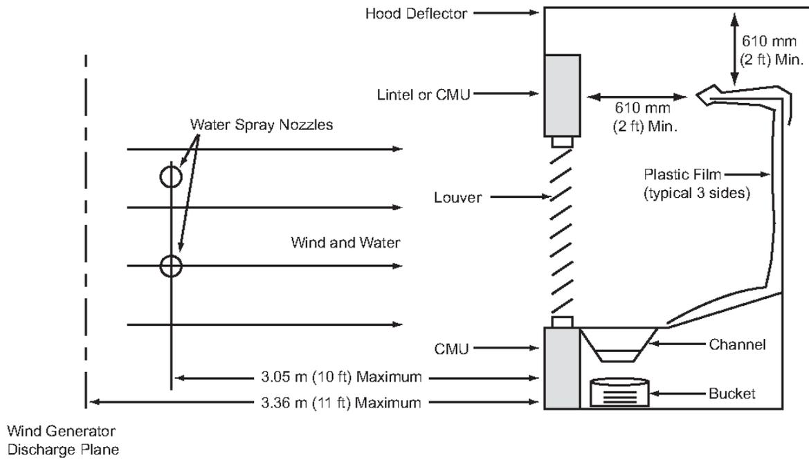
Figure 1 - High Velocity Wind Driven Rain Test Setup
