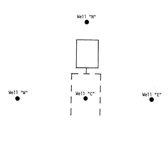
Note: Well "N" will be the north well, etc. Well "C" to well "N", "E", "S", and "W" 50'. It is not necessary that tank and drainfield be oriented in any direction.
