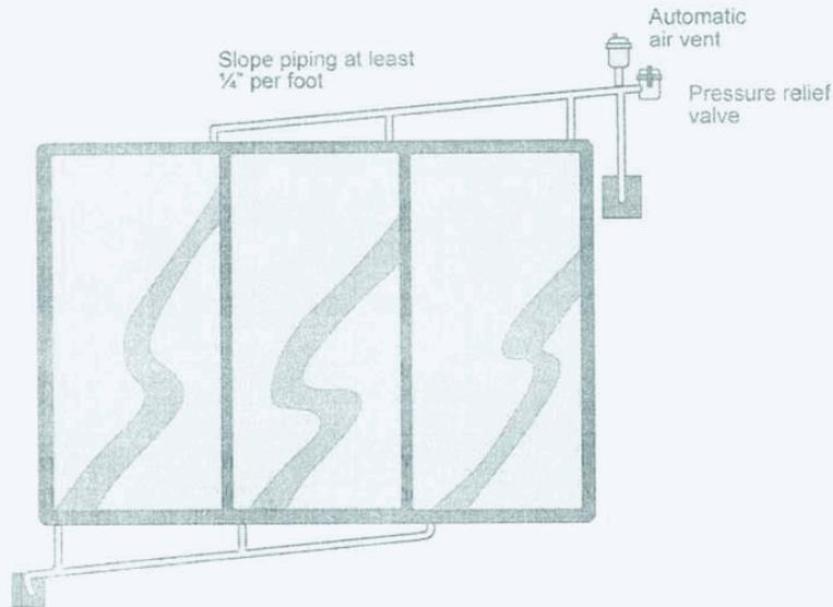
Figure 24 Piped and vented collector array
