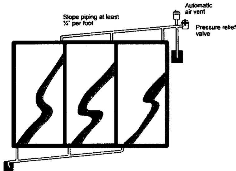
Figure 24 Piped and vented collector array
