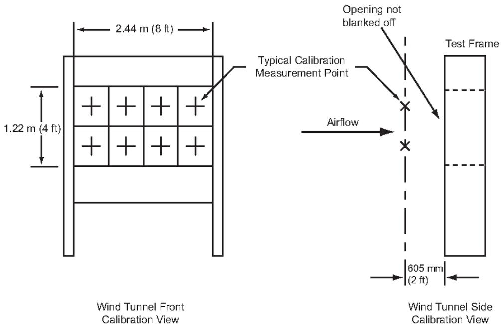
Figure 3 - Wind Stream Calibration Setup
