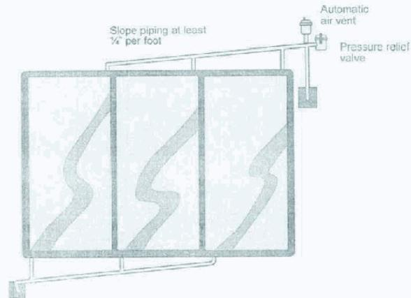
Figure 24 Piped and vented collector array
