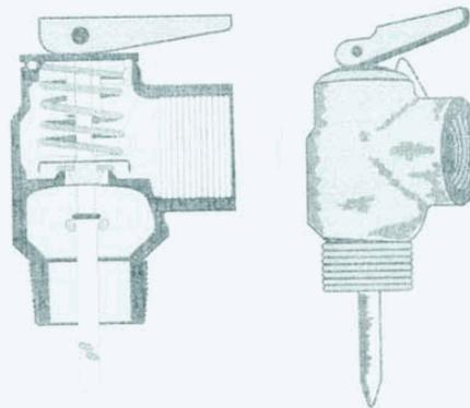
Figure 26 Pressure-temperature relief valve
