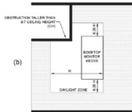
FIGURE C405.2.3.3(3) DAYLIGHT ZONE UNDER A SLOPED ROOFTOP MONITOR
