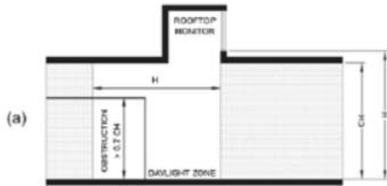
(a) Section view (b) Plan view of daylight zone under a rooftop monitor
