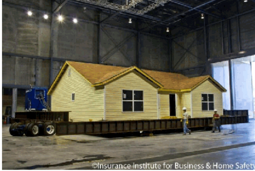
Figure 1-Test duplex moving into the large test chamber at the IBHS Research Center.
