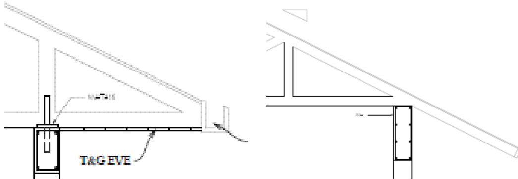
Figure 1. Structural detail of overhang with and without a soffit.
