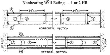
Studs — Channel — shaped 1 5/8 in. wide with 1 3/8 in. legs and 1/4 in. stiffening flanges. Fabricated from No. 25 MSG galv steel. Studs to be cut 1/4 in. less than assembly height.
