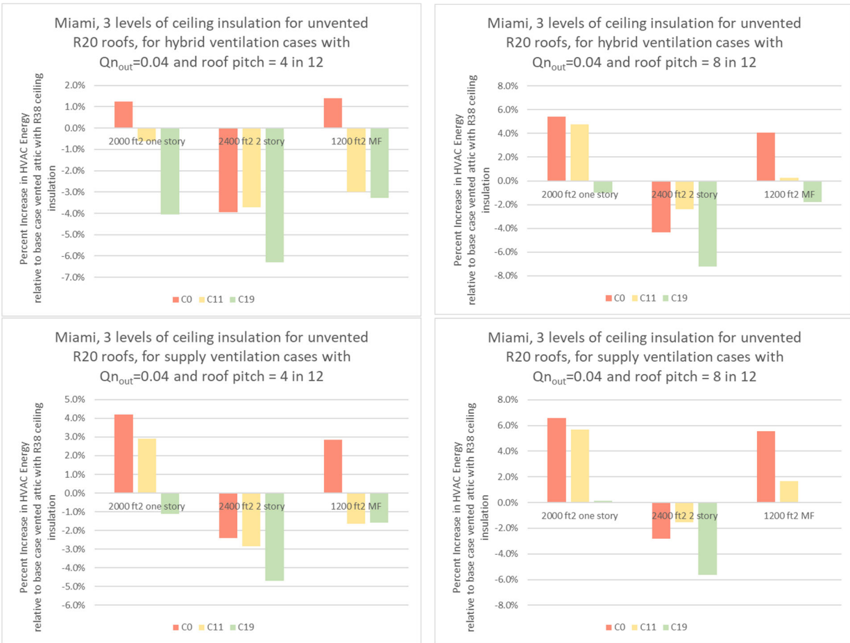
Figure 12. Comparison of three different levels of ceiling insulation for unvented attics relative to base case vented attic with R30 ceiling insulation in Climate Zone 1 for roof pitches of 4 in 12 (charts on left) and 8 in 12 (charts on right) for hybrid ventilation (top charts) and supply-only ventilation (bottom charts).
