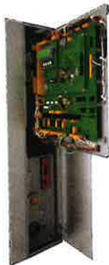
CONTROL PANEL IN DOOR JAMB
