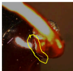
Solder in the cracks of the epoxy/electrode
