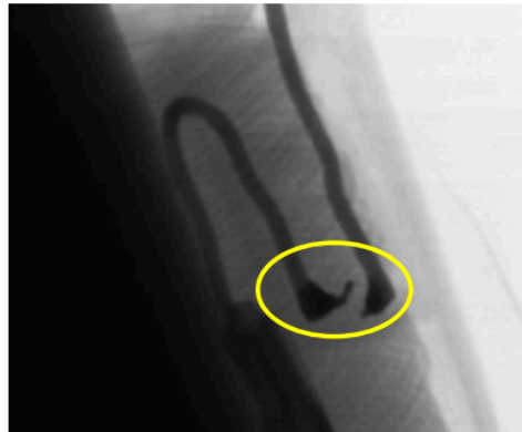
Figure 46. Radiograph of the TCO after the test (sub 23)
