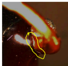
Solder in the cracks of the epoxy/electrode
