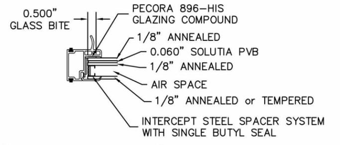
7/8" INSULATED ANNEALED/TEMPERED IMPACT GLASS WITH 0.060" PVB INTERLAYER
