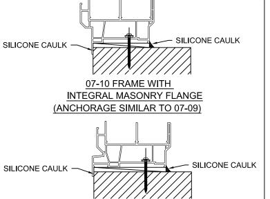
07-20 FRAME WITH INTEGRAL NAILING FIN (REMOVED) & J-CHANNEL (ANCHORAGE SIMILAR TO 07-09)
