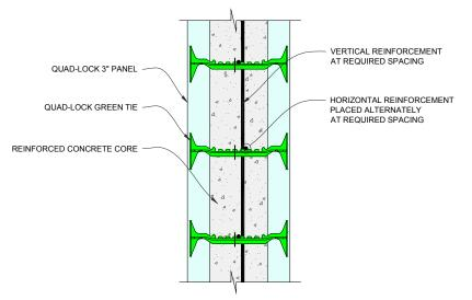
Figure 131: Rebar Placement
