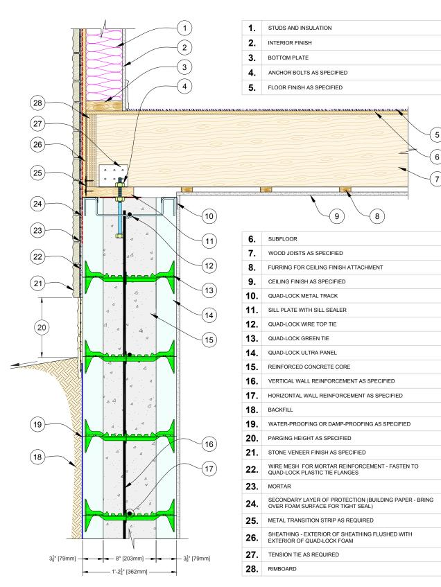
Figure 121: Typical Wall to Floor & Framing Connection
