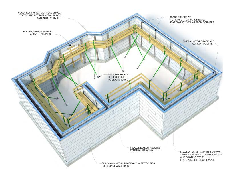
Figure 106: Metal Bracing System
