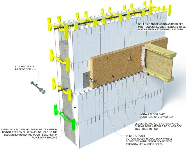
Figure 111: Installation of Floor Ledger Board
