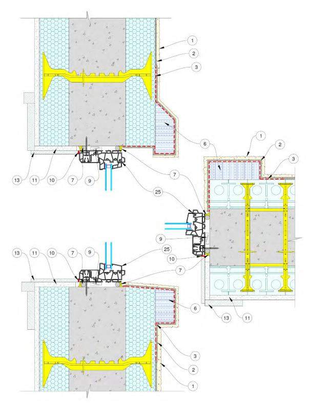
Figure 94: ICF Window Assembly - Direct to concrete, Boxed window centered, EIFS/Stucco lamina
