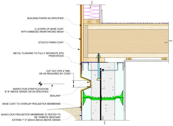
Figure 77: Termite Protection for Foundation Walls
