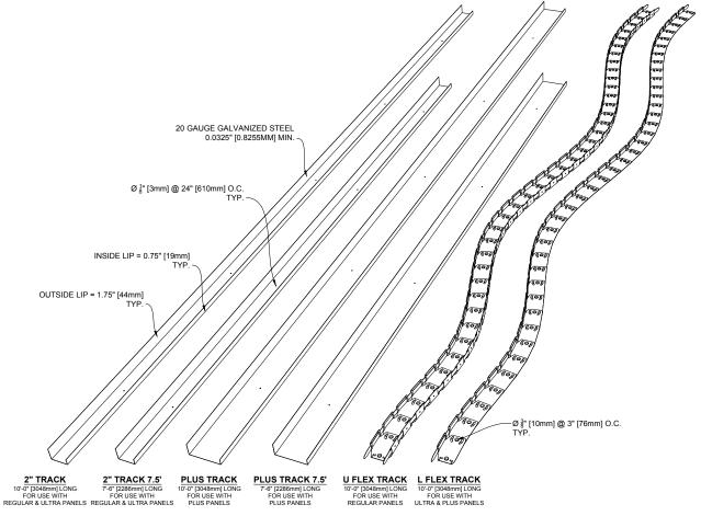
Figure 25: Different Types of Quad-Lock Metal Tracks
