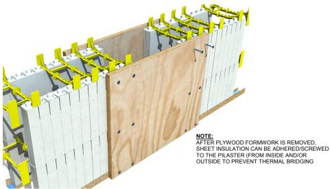
Figure 69: Pilaster formed with Plywood
