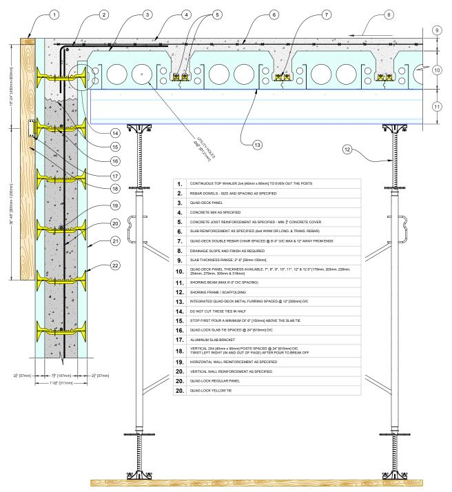
Figure 116: Quad-Deck Concrete Floor Construction Details
