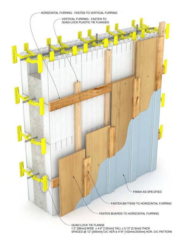
Figure 143: Board & Batten finish with external vertical and horizontal furring strips
