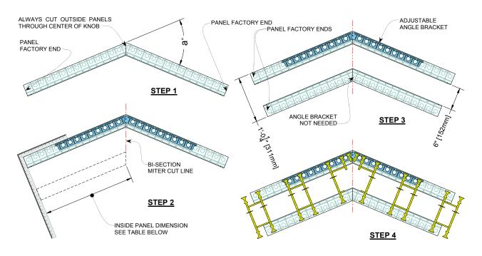
Figure 60: Angled Wall Cutting, Bracket & Tie Placement (Imperial)
