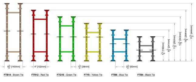
Quad-Lock Ties are molded of High Density Polyethylene (HDPE).
