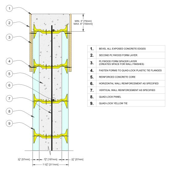
Figure 78: Forming for Solid Wall Cap
