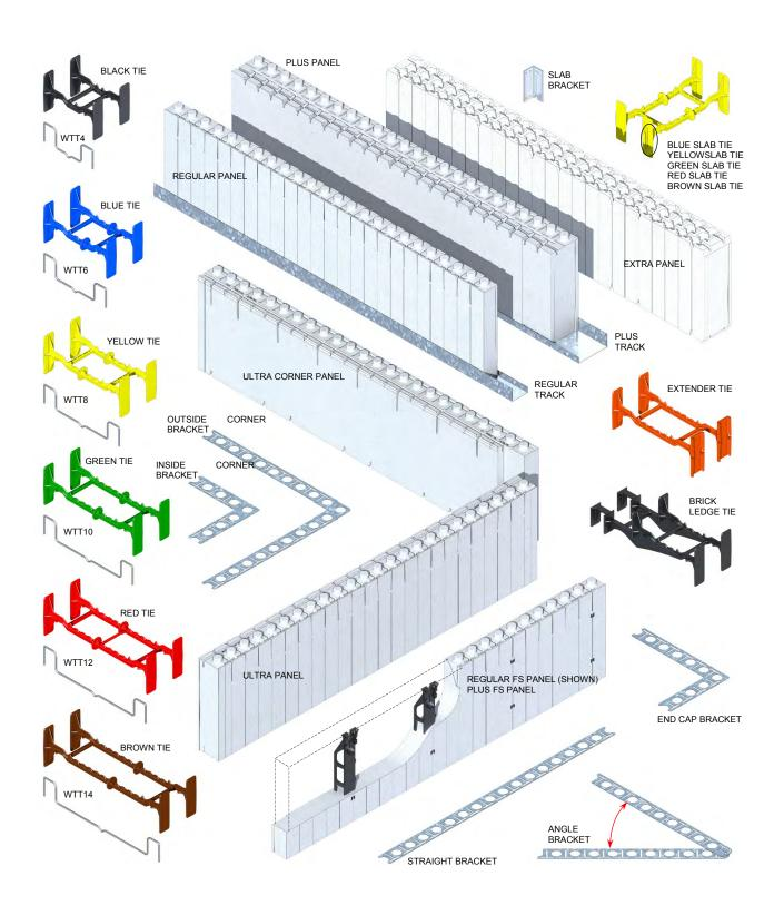
Figure 1: Quad-Lock Components
