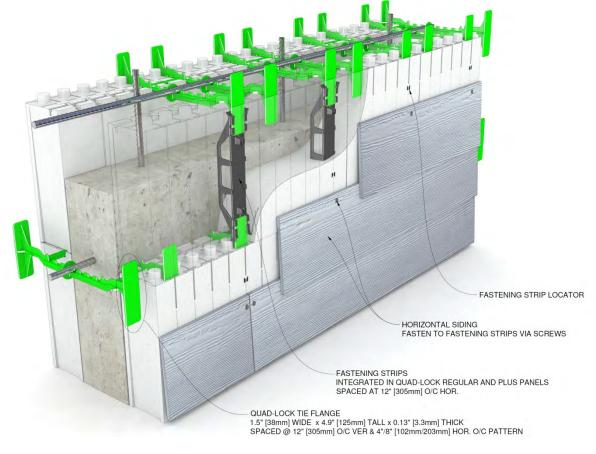
Figure 139: Cladding Details
