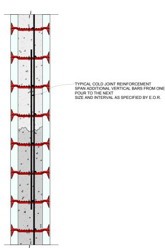
Figure 70: Cold Joint Reinforcement
