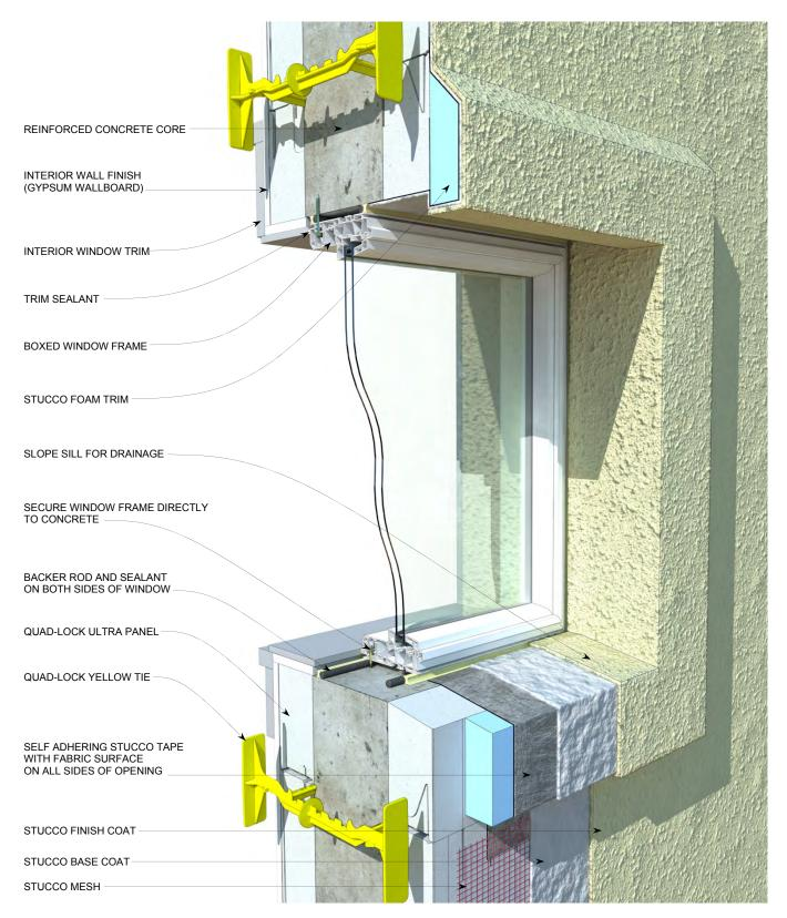
Figure 85: Direct to Concrete Window Assembly
