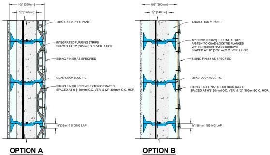
Figure 140: Cladding Detail Options
