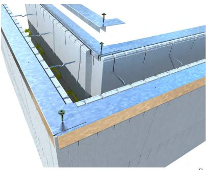
*Figure 52: Overlapping metal track on top of corners*
