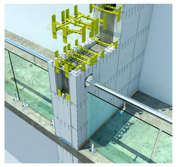
Figure 56: Bulkheads Formed with Quad-Lock End Cap Brackets
