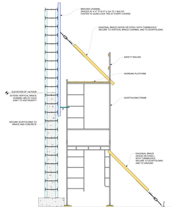
Figure 110: Bracing Tall Walls with Scaffolding
