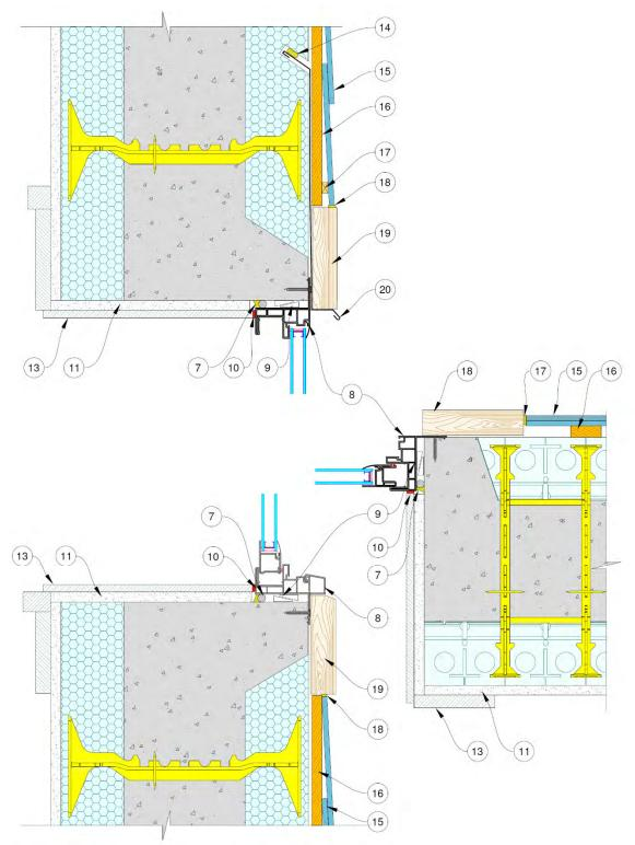
Figure 89: ICF Window Assembly - Direct to concrete, Flanged window flush to exterior, Lapped siding
