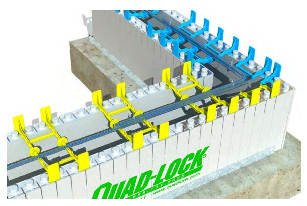
Figure 129: Sample Rebar Placement at Corners & T-Walls
