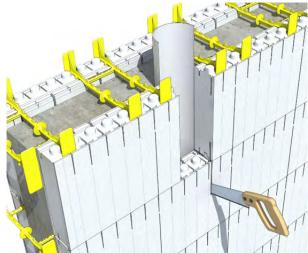
Step 2. Cut out EPS Panels to expose the blocked out area.
