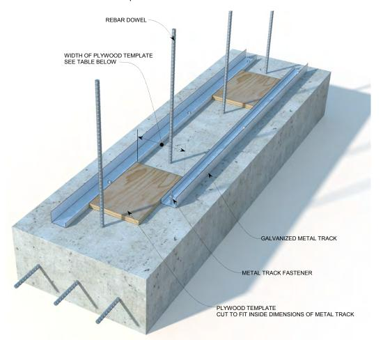
Figure 41: Plywood Templates fit to Wall Dimension
