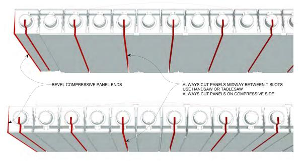
Figure 61: Radius Wall – Panels Cuts
