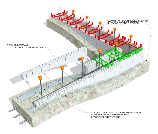
Figure 36: Panels Tapered to Compensate for out-of-level Footing
