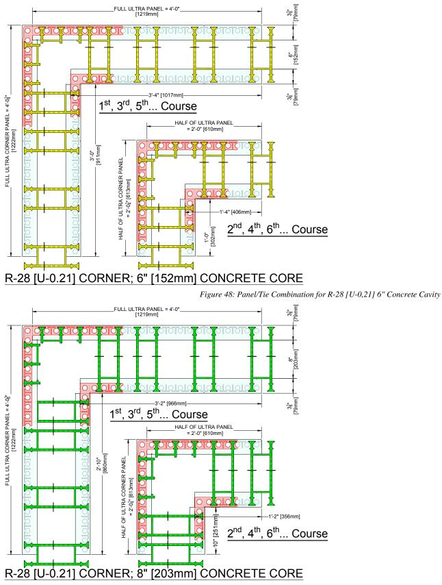
Figure 49: Panel/Tie Combination for R-28 [U-0,21] 8" Concrete Cavity
