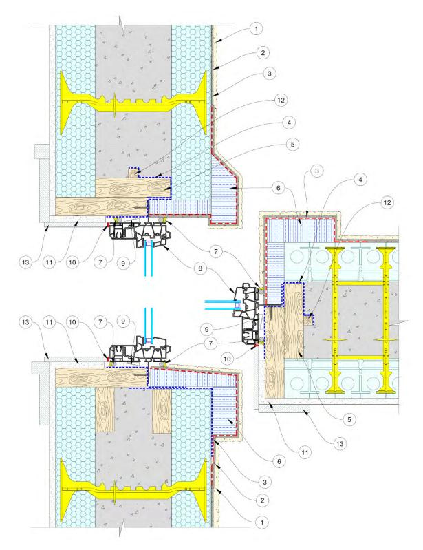
Figure 90: ICF Window Assembly - Wood buck-out, Flanged window centered, EIFS/Stucco lamina
