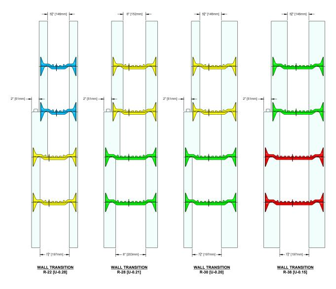
Figure 73: Wall Width Transition using Quad-Lock Plus Panels
