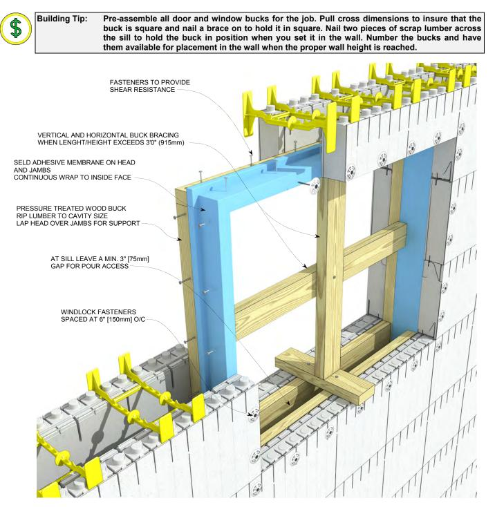
Figure 84: Internal buck-out with water-stop flashing, bracing, and ICF panels fastened to wood members
