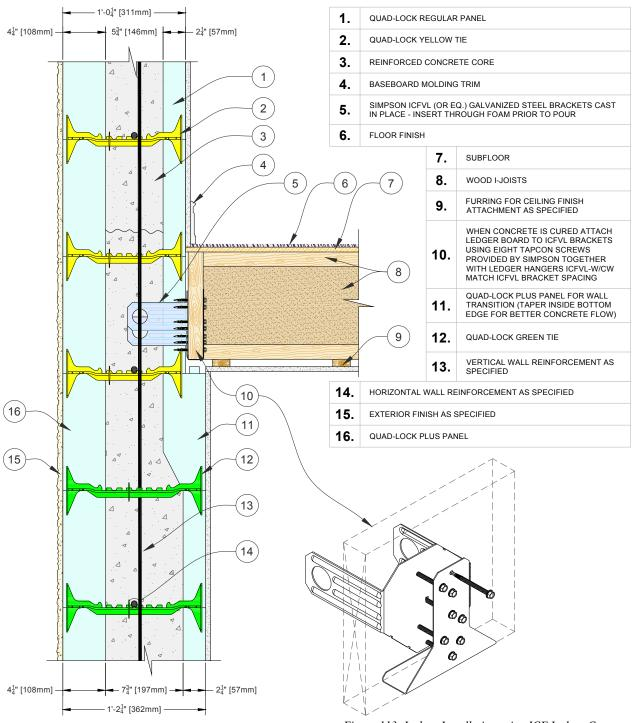
Figure 113: Ledger Installation using ICF Ledger Connectors
