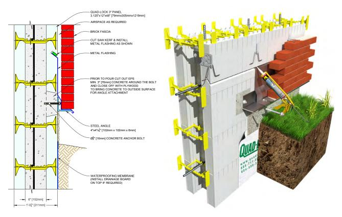
Figure 147: Brick Ledge with Steel Angle Bolted to Concrete
