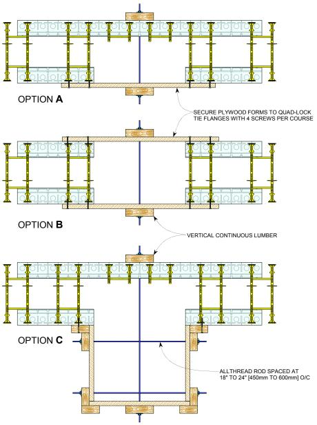
Figure 68: Pilasters formed with Plywood & Threaded Rod
