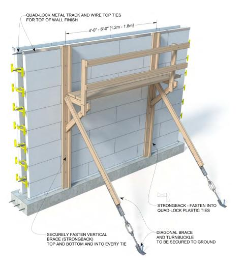
Figure 107: Site Constructed Wood Wall Bracing
