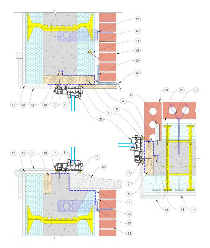
Figure 97: ICF Window Assembly - Wood buck-out, Boxed window centered, Brick veneer
