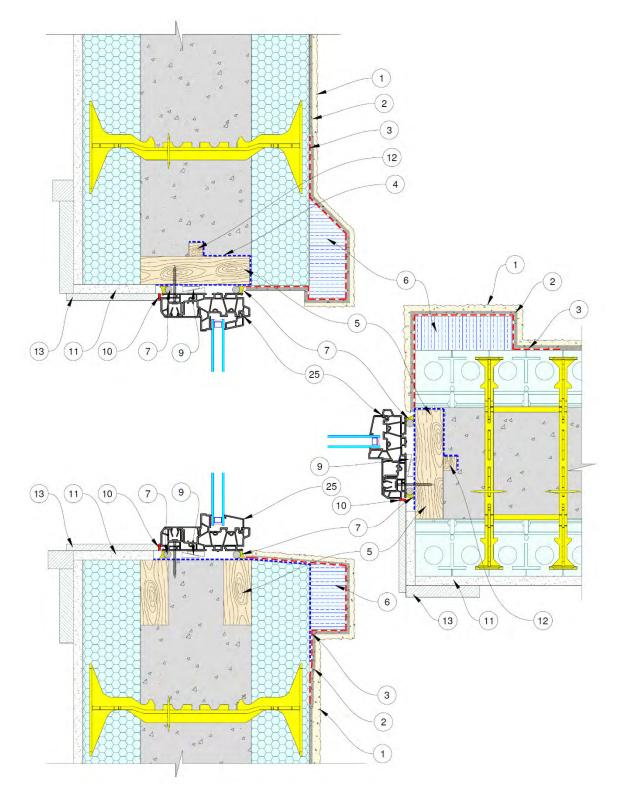
Figure 93: ICF Window Assembly - Wood buck-out, Boxed window centered, EIFS/Stucco lamina
