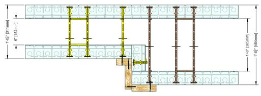
Figure 74: Horizontal (plan view) Wall Width Transition
