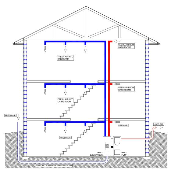
Figure 30: Typical "Passive House" Ventilation System
