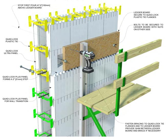
Figure 108: Wall Bracing with Ledger Board in Place
