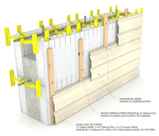
Figure 141: Siding Attachment with external furring strips
