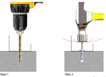
Figure 39: Installation of Hit-Anchors
