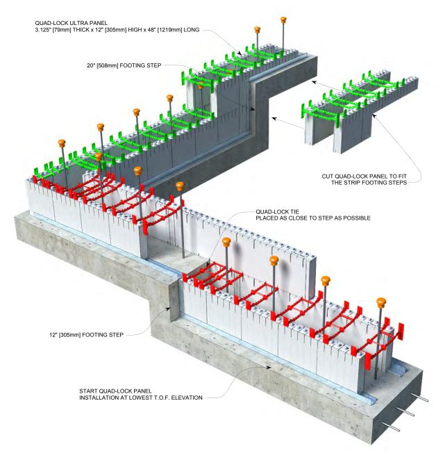
Figure 35: Adapting to Odd Footing Elevations
