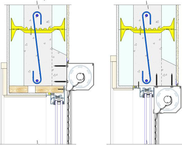
Figure 101: Attachment of Roll-Up Storm Shutter
