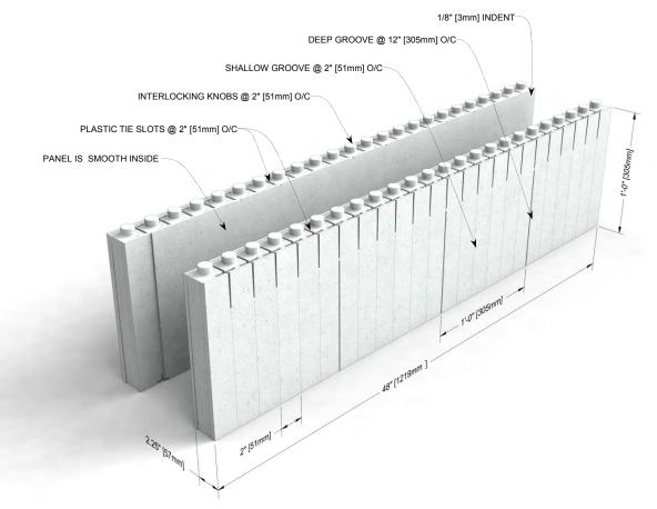
Figure 2: Quad-Lock Regular Panels
