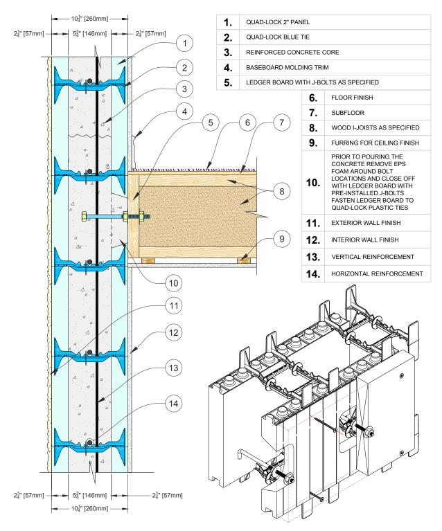
Figure 114: Typical Ledger Board Connection w/ Anchor Bolts
