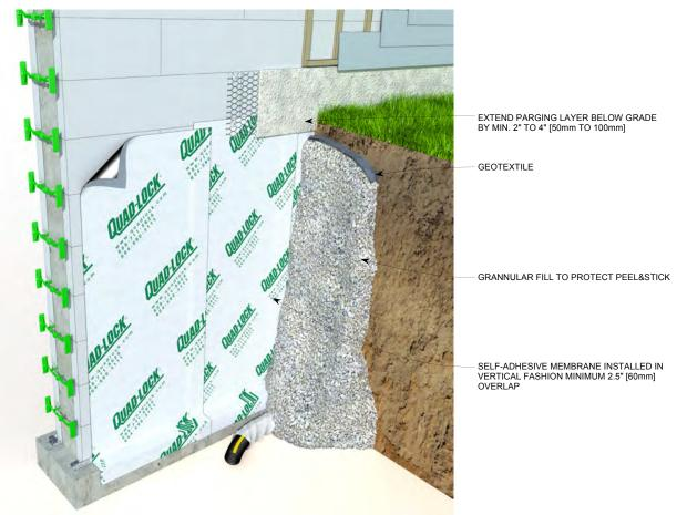
Figure 136: Water Proofing with Peel&Stick
