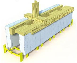
Hybrid Sill - Cut out holes to provide access for pouring
