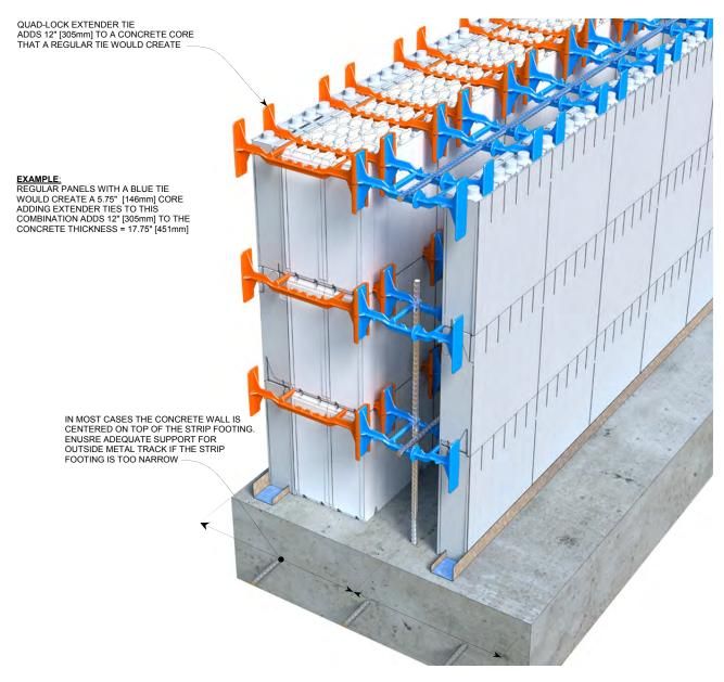
Figure 66: Extender Tie Assembly (20" [508mm] cavity shown)
