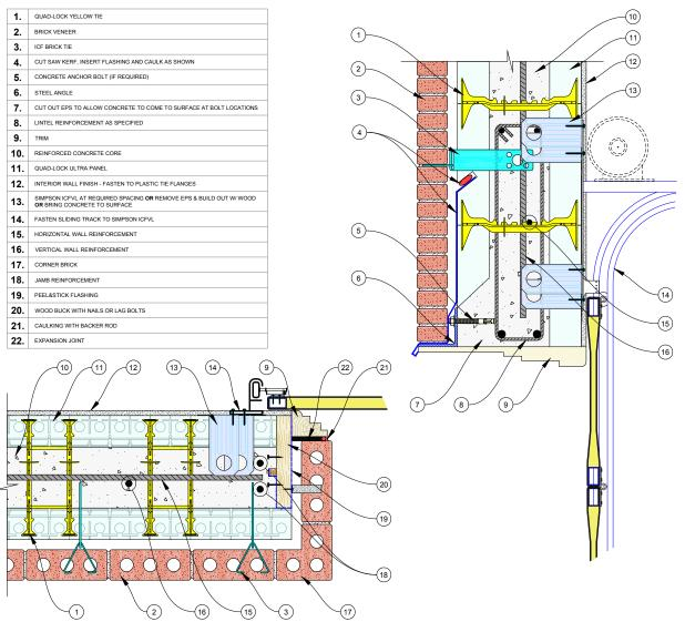
Figure 104: Garage Door at Jamb and Head (Brick Finish)
