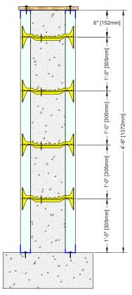
Figure 50: Panels Ripped to Adjust Wall Elevation
