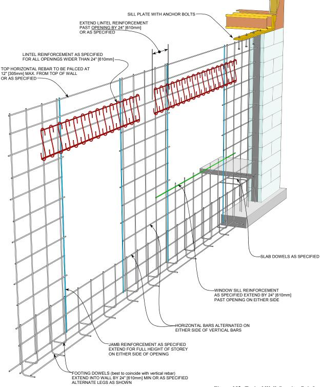
Figure 132: Typical Wall Opening Reinforcement
