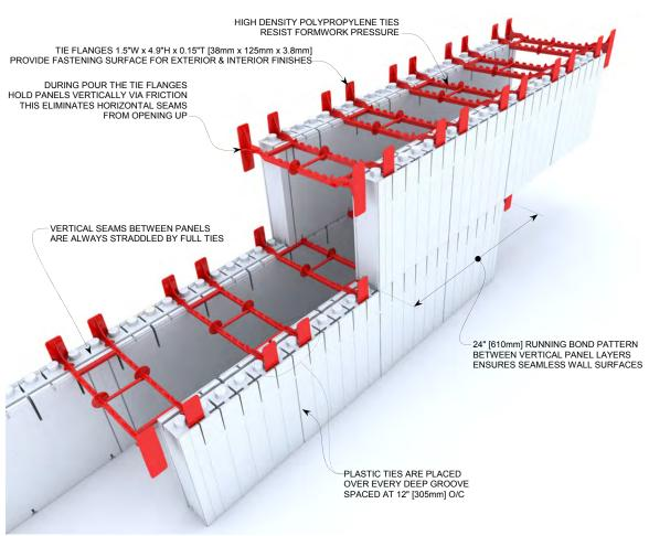
Figure 10: Quad-Lock Ties & Panels
