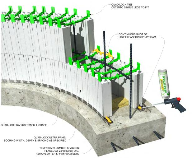
Figure 63: Radius Wall (tight radius)
