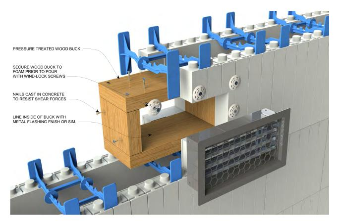
Figure 76: Vent Wall Penetration
