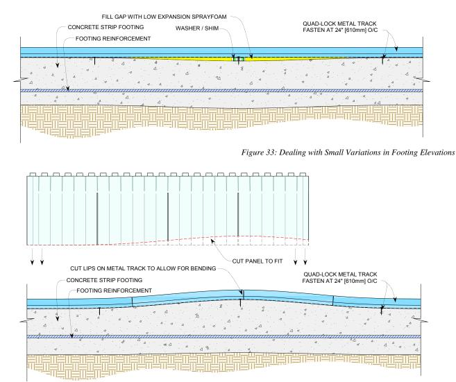
Figure 34: Adapting panels to inconsistencies in footing elevation
