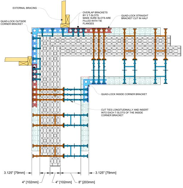
Figure 65: Extender Tie Assembly for Corners
