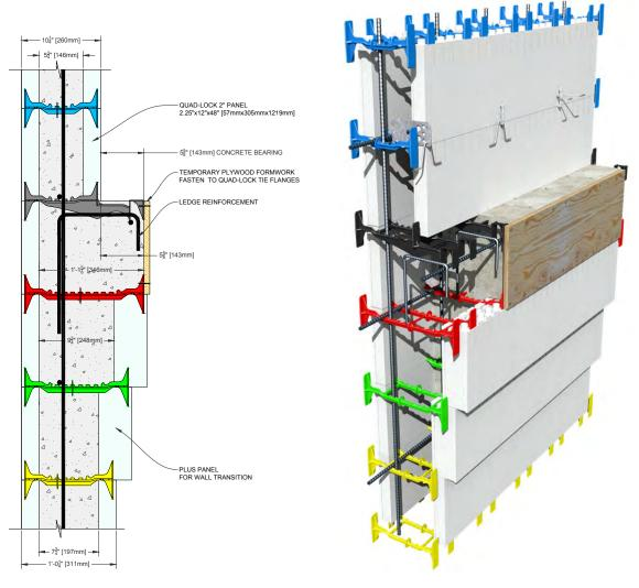
Figure 150: Brick Ledge Formed with Temporary Plywood Forms
