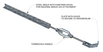
Figure 105: Typical Form Aligner (Turnbuckle) Device
