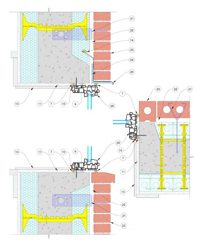
Figure 92: ICF Window Assembly - Direct to concrete, Boxed window flush, Brick veneer
