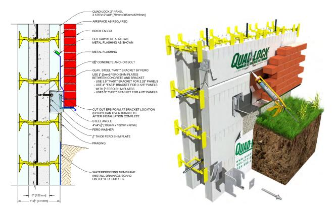
Figure 149: Steel Angle Brick Ledge Supported with Fero Brackets
