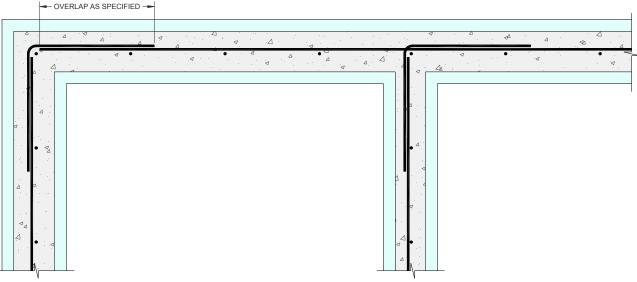
Figure 130: Typical Lap Patterns at Corners & T-Walls
