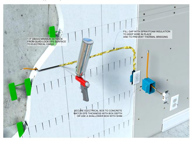
Figure 160: Installation of Electrical Boxes and Wiring
