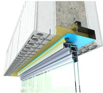
Figure 80: Internal Wood Buck-out in position between ICF panels
