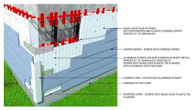
Figure 145: Corner Trim Attachment with Siding Directly Applied to Quad-Lock
