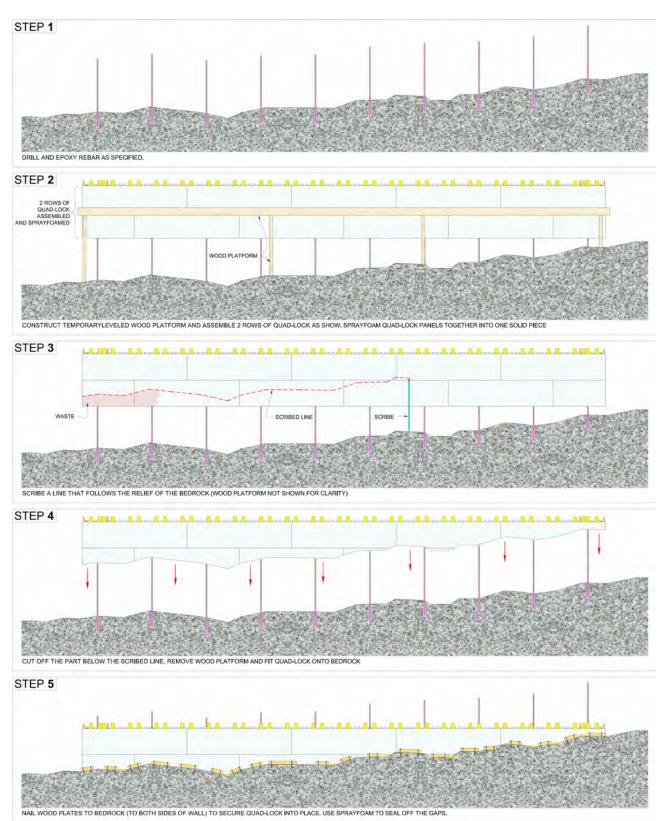
Figure 40: Quad-Lock Wall Installation on Bedrock
