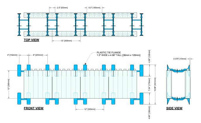
Figure 12: Tie Layout Dimensions
