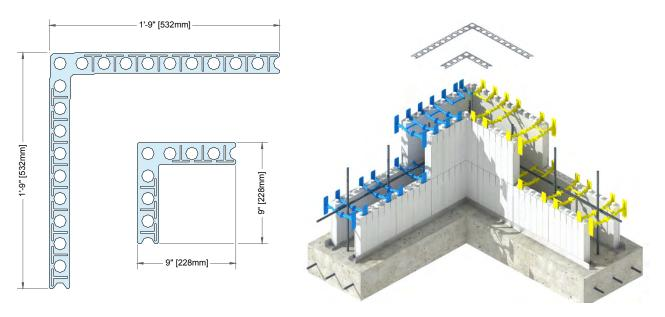
Figure 17: Inside and Outside Corner Brackets
