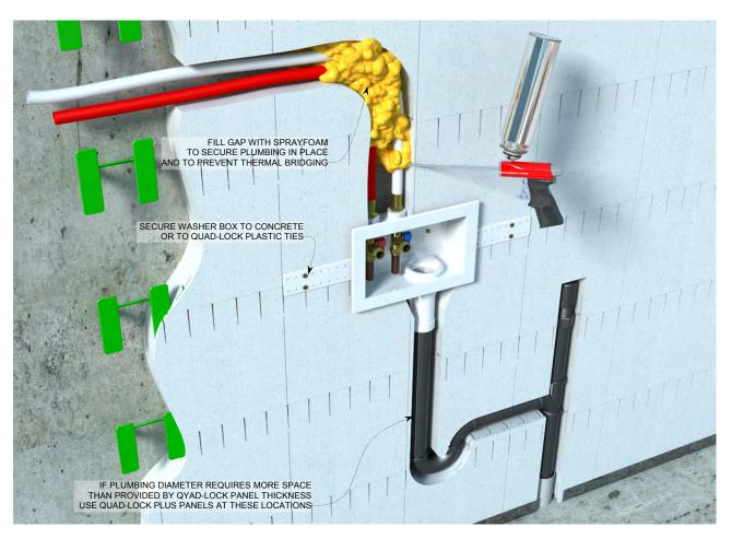
Figure 161: Plumbing Installation (After-Pour Method)
