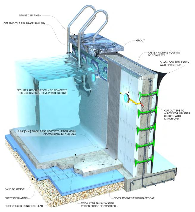
Figure 163: Typical Swimming Pool Wall section
