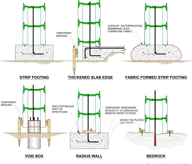
Figure 37: Typical Bottom of Wall Details
