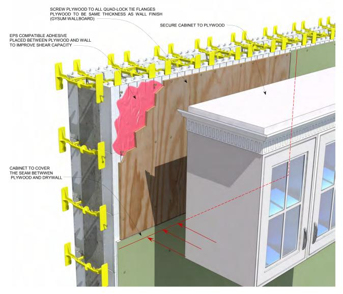
Figure 156: Attaching Heavy Items using Plywood behind Cabinets
