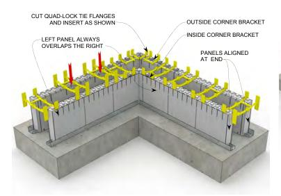
MAINTAIN 2 FOOT [609mm] RUNNING BOND PATTERN BY PLACING THE PANELS OVER TOP OF A VERTICAL PANEL JOINT OF THE ROW BELOW
