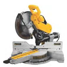
Figure 43: Recommended Tools for Cutting EPS Panels
