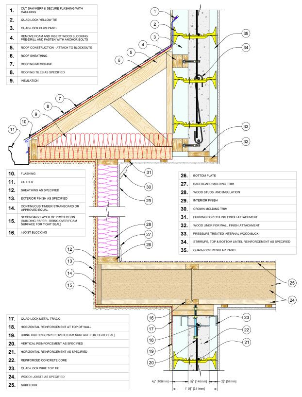
Figure 123: Cantilevered Joist Connection
