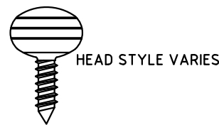
11 THUMB SCREW SCALE: FULL SIZE
