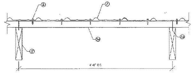
1. **Metal Roof Deck Panels\*** — No. 29 MSG min coated steel. Max panel width 36 in Rib height max 3/4 in. Panels continuous over two or more spans. Panels to overlap 6 in. at endlaps and must occur adjacent to a support when plywood decking (Item 3) is not used. A bead of sealant may be used at panel endlaps and sidelaps.
