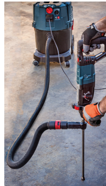
Bosch / Simpson Strong-Tie DXS drill bit used with the vacuum dust extraction system described in Section 3.2.3.2
