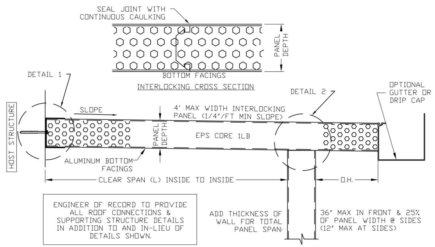
ENGINEER OF RECORD TO PROVIDE ALL ROOF CONNECTIONS & SUPPORTING STRUCTURE DETAILS IN ADDITION TO AND IN-LIEU OF DETAILS SHOWN.
