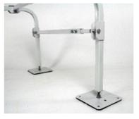
7. Attach the two stability arms to the sides of the stand. Insert one 3/8"-16 x 1 3/4" Hex Bolt, 3/8" Split Washer and 3/8" Nut to hole on face of arm.
