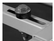
7. Mount unit to stand and insert in slot one 3/8"-16 x 1 1/2" bolt, two 3/8" galvanized washers, one rubber washer, one 3/8" split washer and one 3/8" nut.
