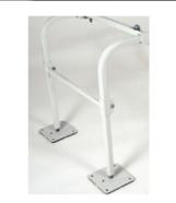
6. Attach the two stability arms to the sides of the stand. Insert one 3/8"-16 x 1 3/4" Hex Bolt, 3/8" Split Washer and 3/8" nut to hole on face of arm.
