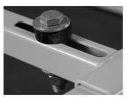
7. Mount unit to stand and insert in slot one 3/8"-16 x 1 1/2" bolt, two 3/8" galvanized washers, one rubber washer, one 3/8" split washer and one 3/8" nut.
