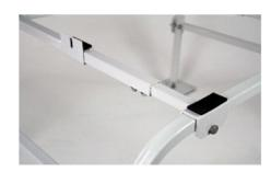
6. Attach arms to completed U-Bars. Insert one 3/8"-16 x 1 3/4" Hex Bolt, 3/8" Split Washer and 3/8" Nut to hole on face of arm.
