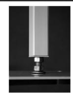
Screw on the adjustment U-Bar until foot is locked in place.
