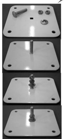
1. Insert 3/8"-16x2" Carriage Bolt through bottom of foot.
