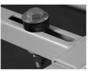
7. Mount unit to stand and insert in slot one 3/8"-16 x 1 ½" Bolt, two 3/8" Galvanized Washers, one Rubber Washer, one 3/8" Split Washer and one 3/8" Nut.
