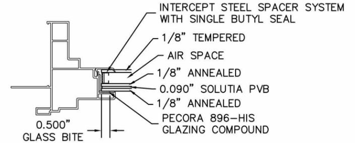
7/8" INSULATED TEMPERED/ANNEALED IMPACT GLASS WITH 0.090" PVB INTERLAYER
