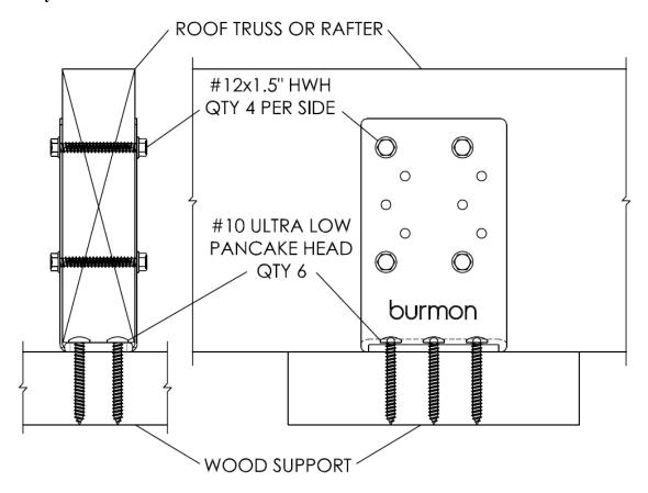
**Material Types:** Roof truss/rafter is Spruce/Pine/Fir wood (G=0.42 min.). Evaluated wood supports by others are untreated engineered LVL wood members (G=0.50 min.) for single top plate or sawn lumber untreated wood (G=0.55 min.) for double top plate. Wood supports may be part of wood construction or be installed by others over ICF/concrete/masonry construction. Attachment of wood supports to ICF/concrete/masonry is by others and beyond the scope of this evaluation.
