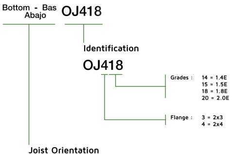
Each TRIFORCE® open joist is marked to indicate a bottom flange. In order to achieve maximum shear capacity, the joist should be installed with proper orientation.
