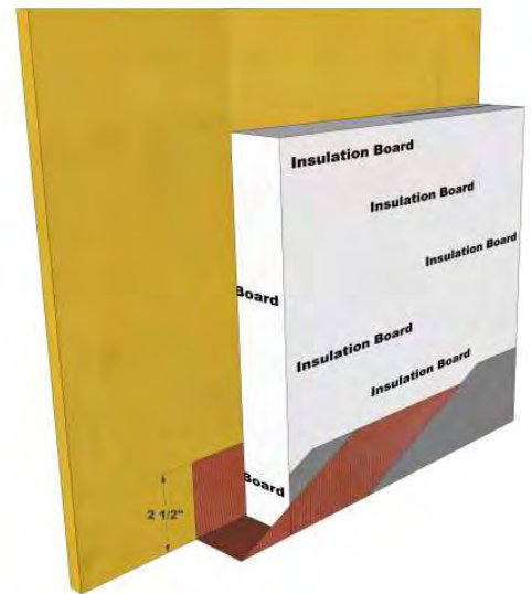
Typical Backwrap Condition
