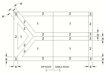
a: 10% OF LEAST HOIZONTAL DIMENSION OR 0.4h, WHICHEVER IS SMALLER, BUT NOT LESS THAN EITHER 4% OF LEAST HORIZONTAL DIMENSION OR 3FT (0.9M).
