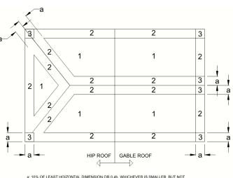
a: 10% OF LEAST HOIZONTAL DIMENSION OR 0.4h, WHICHEVER IS SMALLER, BUT NOT LESS THAN EITHER 4% OF LEAST HORIZONTAL DIMENSION OR 3FT (0.9M). OR AS DETERMINED BY DESIGN OR OTHER APPLICABLE CODE.
