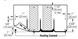
Figure 17-5: When installing Grand Manor Shangles on steep slopes, use **seven** nails and three spots of asphalt roofing cement.
