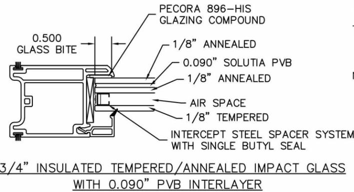
3/4" INSULATED TEMPERED/ANNEALED IMPACT GLASS WITH 0.090" PVB INTERLAYER
