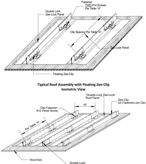
Typical Roof Assembly with Zee-Clips Isometric View
