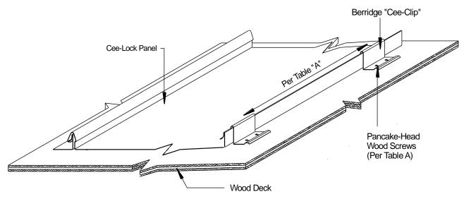
Typical Roof Assembly with Berridge "Cee-Clip" Panel Clip - Isometric View
