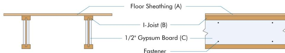
**(A) Floor Sheathing:** Materials and installation must be per 2018, 2015 or 2012 IRC Section R503
