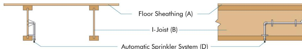
**(D) Automatic Sprinkler System:** System in accordance with Section P2904 of the 2018 or 2015 or 2012 IRC, NFPA 13D, or other equivalent sprinkler system. **Note:** Per 2018 or 2015 or 2012 IRC Section P2904, partial residential sprinkler systems are permitted to be installed only in buildings not required to be equipped with a residential sprinkler system. Check with the local building official for specific jurisdictional requirements.
