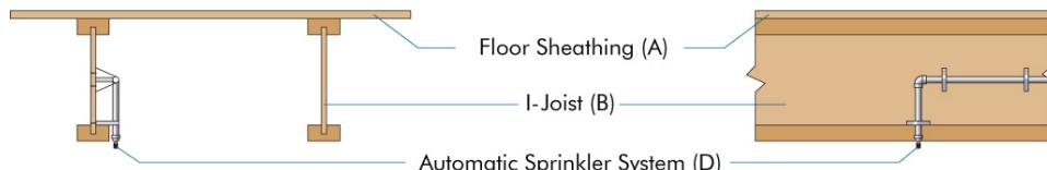
**(D) Automatic Sprinkler System:** System in accordance with Section P2904 of the 2018, 2015 or 2012 IRC, NFPA 13D, or other equivalent sprinkler system. **Note:** Per 2018, 2015 or 2012 IRC Section P2904, partial residential sprinkler systems are permitted to be installed only when the entire dwelling unit is not required to be equipped with a residential sprinkler system. Check with the local building official for specific jurisdictional requirements.
