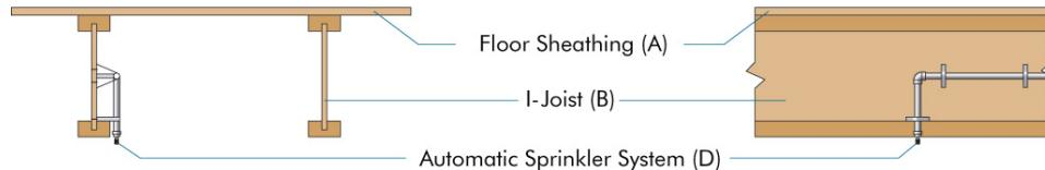
(D) Automatic sprinkler system: System in accordance with Section P2904 of the 2018, 2015 and 2012 IRC, NFPA 13D, or other equivalent sprinkler systems. Note: Per 2018, 2015 or 2012 IRC Section P2904, partial residential sprinkler systems are permitted to be installed only in buildings not required to be equipped with a residential sprinkler system. Check with the local building official for specific jurisdictional requirements.
