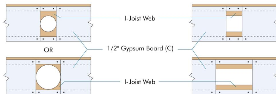
**Note:** At hole location, fasteners must be installed 1 inch from the edge of the gypsum board and horizontally spaced a distance equivalent to the hole width/diameter plus 2 inches. Maximum fastener spacing shall be no more than 8" on gypsum board above and below the hole.
