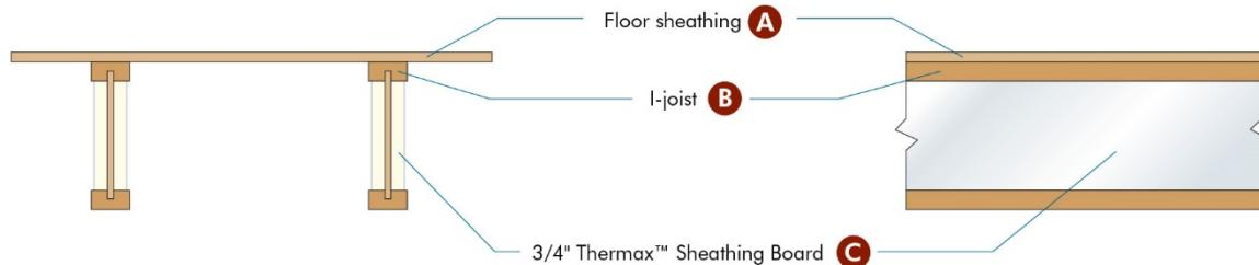
(A) Floor sheathing: Materials and installation must be per Section R503 of the 2018, 2015 or 2012 IRC.
