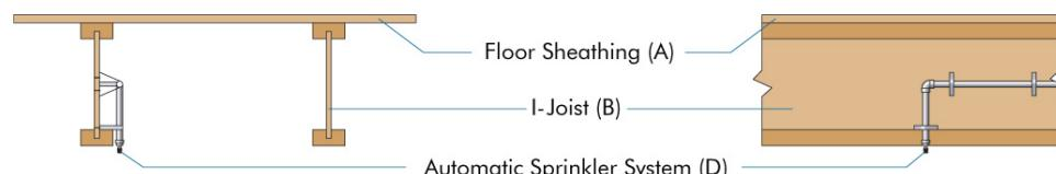
**(D) Automatic Sprinkler System:** System in accordance with Section P2904 of the 2018, 2015 IRC or 2012 IRC, NFPA 13D, or other equivalent sprinkler system. **Note:** Per 2018, 2015 or 2012 IRC Section P2904, partial residential sprinkler systems are permitted to be installed only in buildings not required to be equipped with a residential sprinkler system. Check with the local building official for specific jurisdictional requirements.
