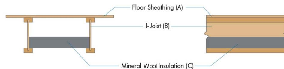
**(A) Floor Sheathing:** Materials and installation must be per 2018, 2015 or 2012 IRC Section R503.
