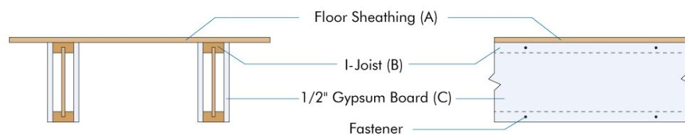
(A) **Floor Sheathing:** Materials and installation must be per 2018, 2015 or 2012 IRC Section R503.
