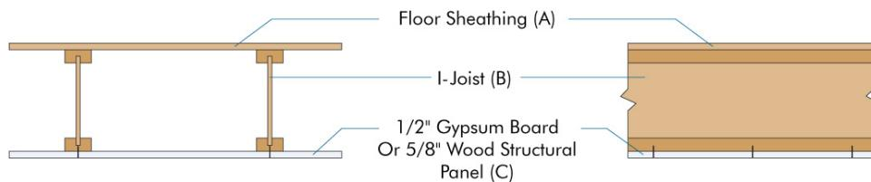
(A) Floor Sheathing: Materials and installation must be per 2018, 2015 or 2012 IRC Section R503.
