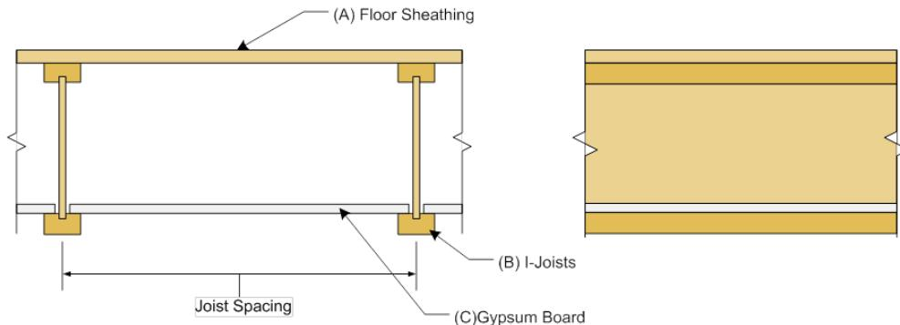
**(A) Floor Sheathing:** Materials and installation must be per 2018, 2015 or 2012 IRC Section R503.
