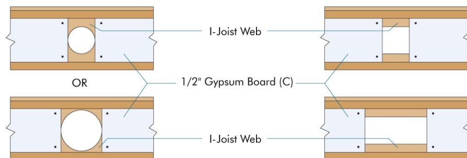
**Note:** At hole location, fasteners must be installed 1 inch from the edge of the gypsum board and horizontally spaced a distance equivalent to the hole width/diameter plus 2 inches.
