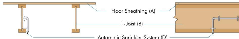
**(D) Automatic Sprinkler System:** System in accordance with Section P2904 of the 2018, 2015 or 2012 IRC, NFPA 13D, or other equivalent sprinkler system. **Note:** Per 2018, 2015 or 2012 IRC Section P2904, partial residential sprinkler systems are permitted to be installed only in buildings not required to be equipped with a residential sprinkler system. Check with the local building official for specific jurisdictional requirements.
