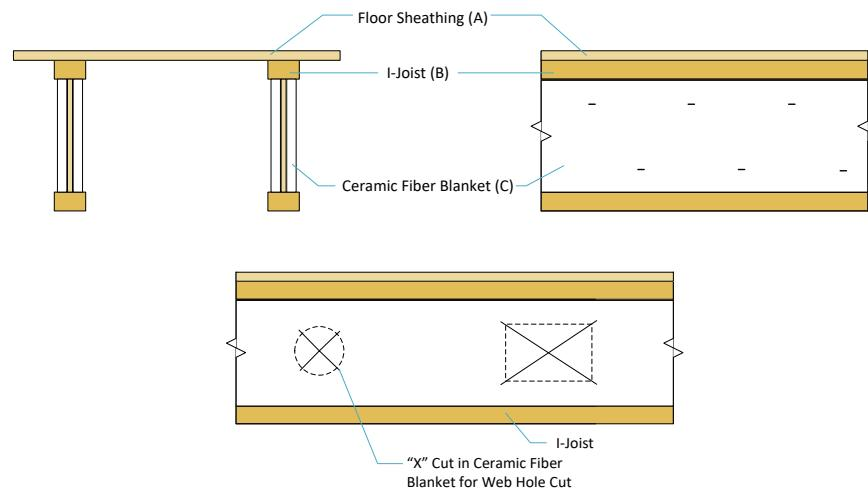
**(A) Floor Sheathing:** Materials and installation must be per 2018, 2015 IRC or 2012 IRC Section R503.
