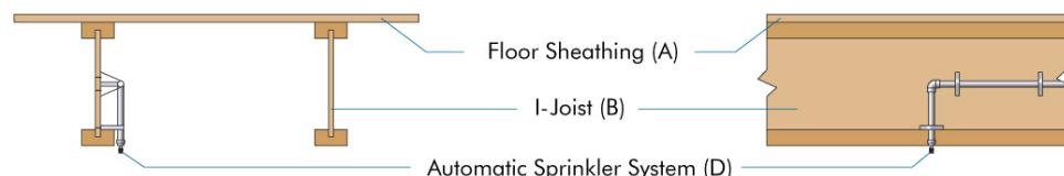
(D) **Automatic Sprinkler System:** System in accordance with Section P2904 of the 2018, 2015 or 2012 IRC, NFPA 13D, or other equivalent sprinkler system. **Note:** Per 2018 or 2015 IRC or 2012 IRC Section P2904, partial residential sprinkler systems are permitted to be installed only in buildings not required to be equipped with a residential sprinkler system. Check with the local building official for specific jurisdictional requirements.
