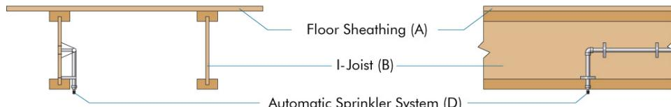
(D) Automatic Sprinkler System: System in accordance with Section P2904 of the 2018, 2015 or 2012 IRC, NFPA 13D, or other equivalent sprinkler system. Note: Per 2018, 2015 or 2012 IRC Section P2904, partial residential sprinkler systems are permitted to be installed only in buildings not required to be equipped with a residential sprinkler system. Check with the local building official for specific jurisdictional requirements.
