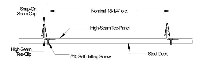
Typical Assembly Profile View (Typical Fastening Pattern Across Width)
