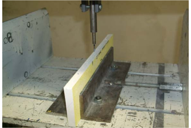
Typical Core End & Edge Hardness Test Set-up
