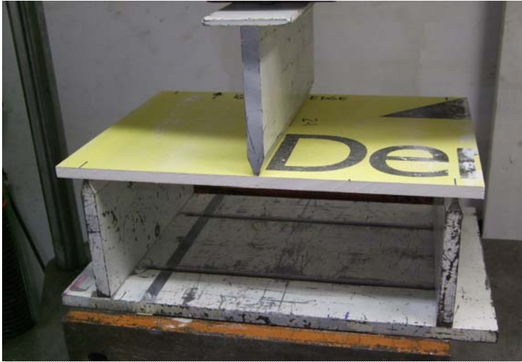
Typical Flexural Test Set-up
