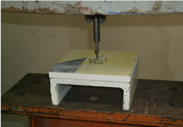
Typical Nail Pull Resistance Test Set-up
