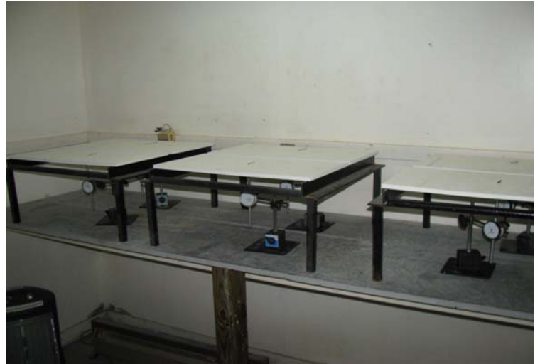
Typical Humidified Deflection Test Set-up
