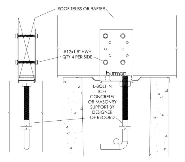
**Material Types:** Roof truss/rafter is Spruce/Pine/Fir wood (G=0.42 min.). ICF, Concrete, and/or Masonry construction and reinforcement is by others and beyond the scope of this evaluation.
