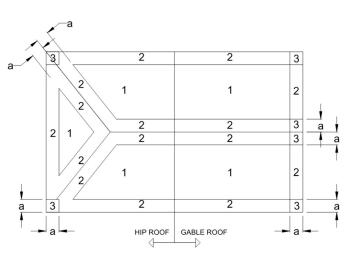
a: 10% OF LEAST HOIZONTAL DIMENSION OR 0.4h, WHICHEVER IS SMALLER, BUT NOT LESS THAN EITHER 4% OF LEAST HORIZONTAL DIMENSION OR 3FT (0.9M).
