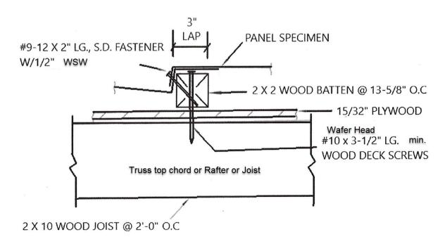
Section Attachment at wood joist locations = 24 in oc
