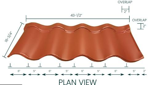
ALL FASTENERS #9 X 2" LG. S.D. FASTENERS WITH METAL
