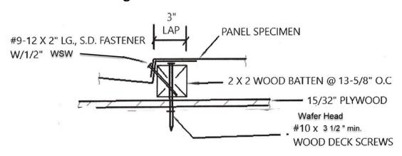
Section Attachment at Plywood deck only locations = 24 in oc
