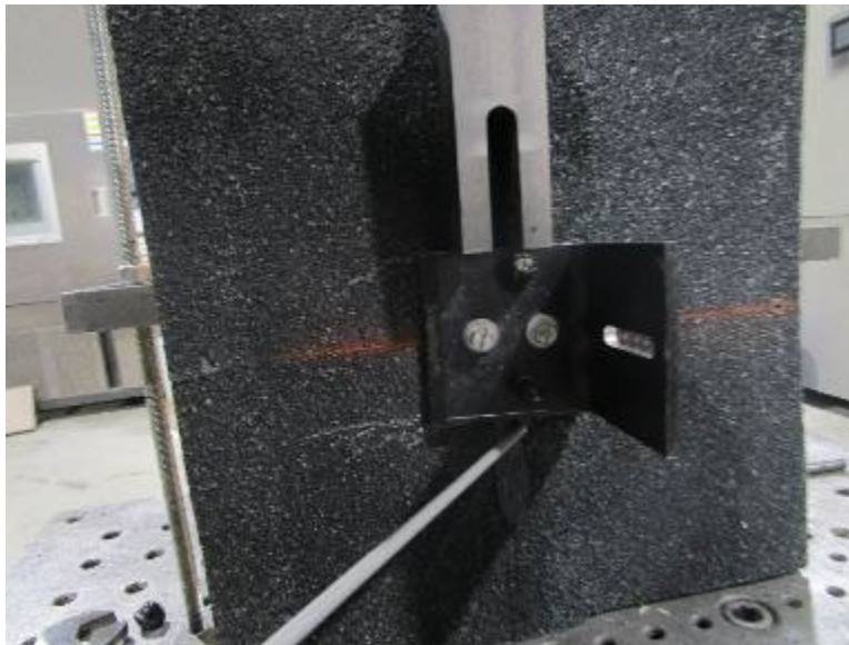
Photo No. 3 Shear Parallel to the Flange
